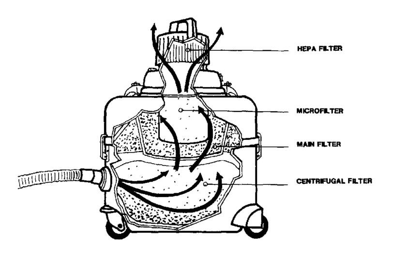
Figure 2 HEPA-Vacuum Schematic
