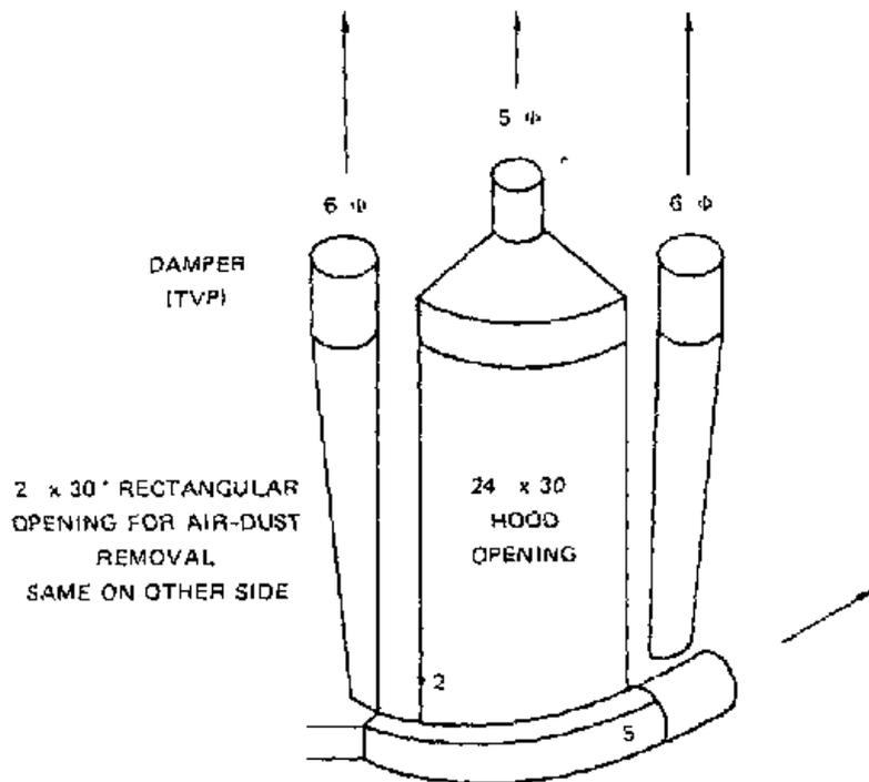
NOTE All four above units to be mounted on hood around the 24 x 30 opening
