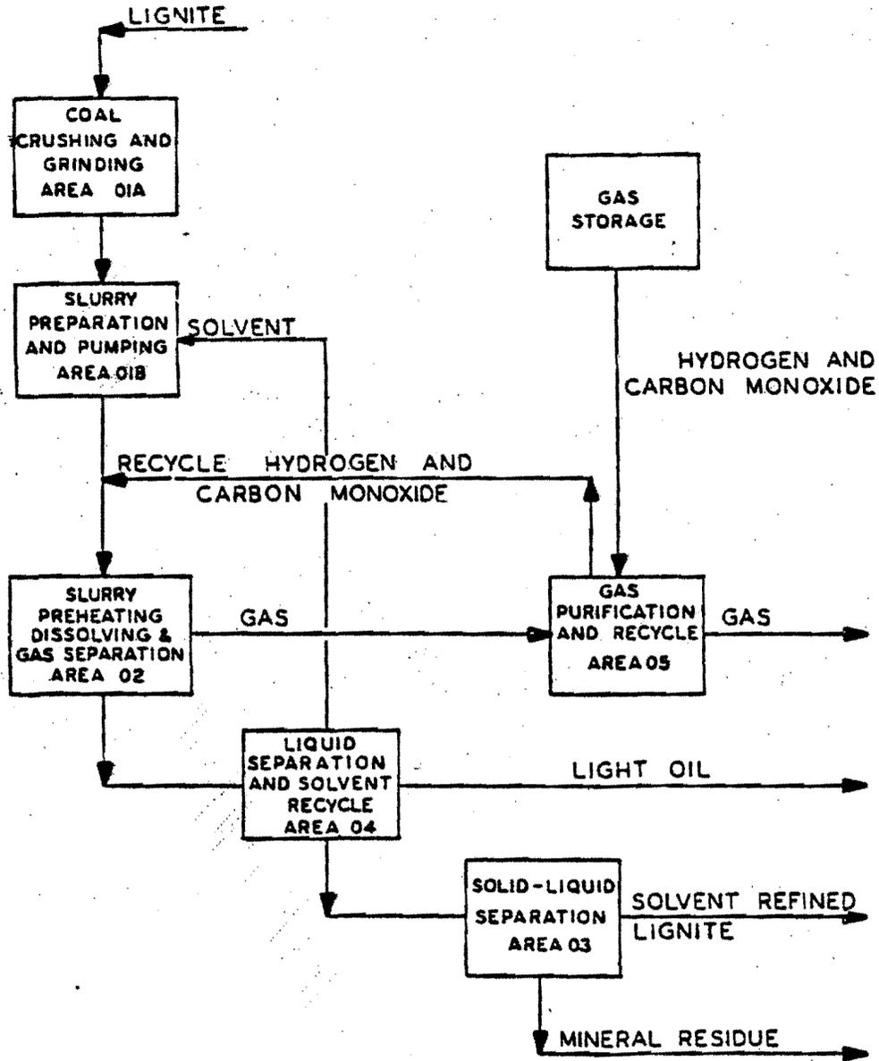
**FIGURE 1** - Simplified Block - Flow Diagram<sup>a</sup> of the Solvent Refined Lignite Process Development Unit (SRL PDU), University of North Dakota, Grand Forks
