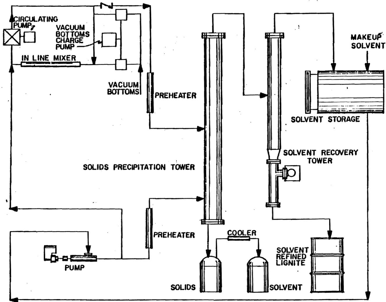
FIGURE 2 - Diagram of the Solid-liquid Separation Unit<sup>a</sup>
