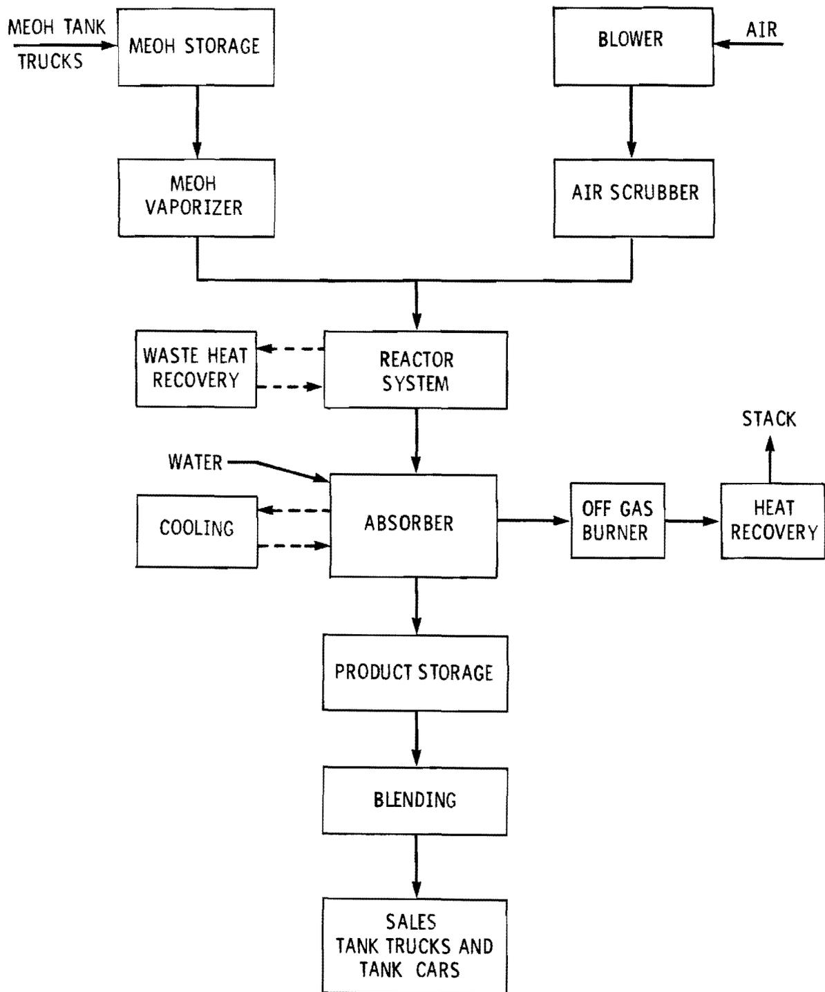
Figure 2. Formaldehyde process - block flow diagram.
