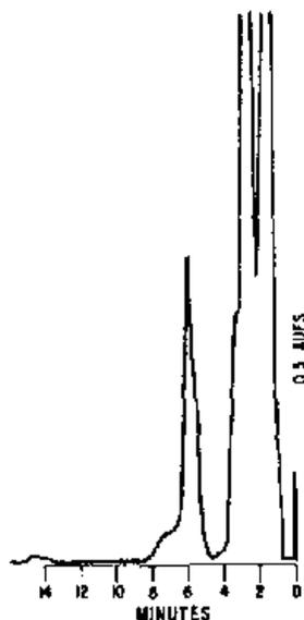
Figure 3 HPLC chromatogram for a field sample at a location where formaldehyde is used as a raw material. The sample was determined to represent 0.85 ppm formaldehyde in air
