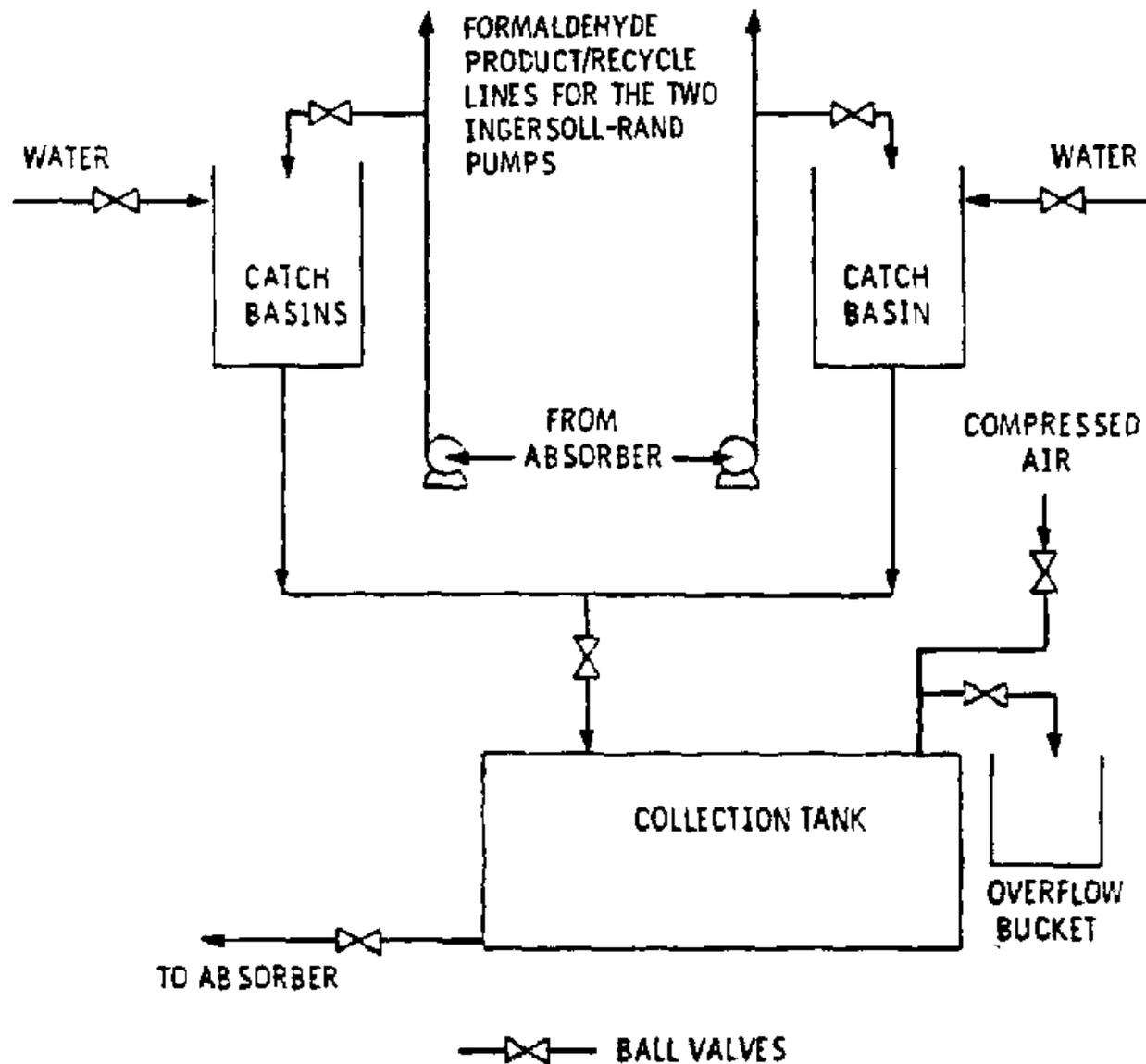
Figure 4. Schematic of process sampling/purge collection system.
