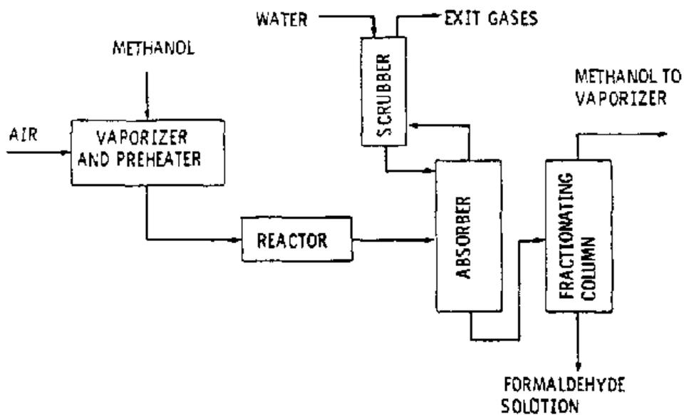
Figure 3. Formaldehyde production process using a silver catalyst [21].
