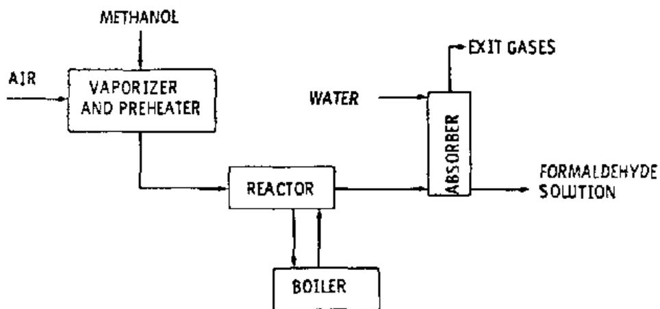
Figure 2. Formaldehyde production process using a metal oxide catalyst [20].
