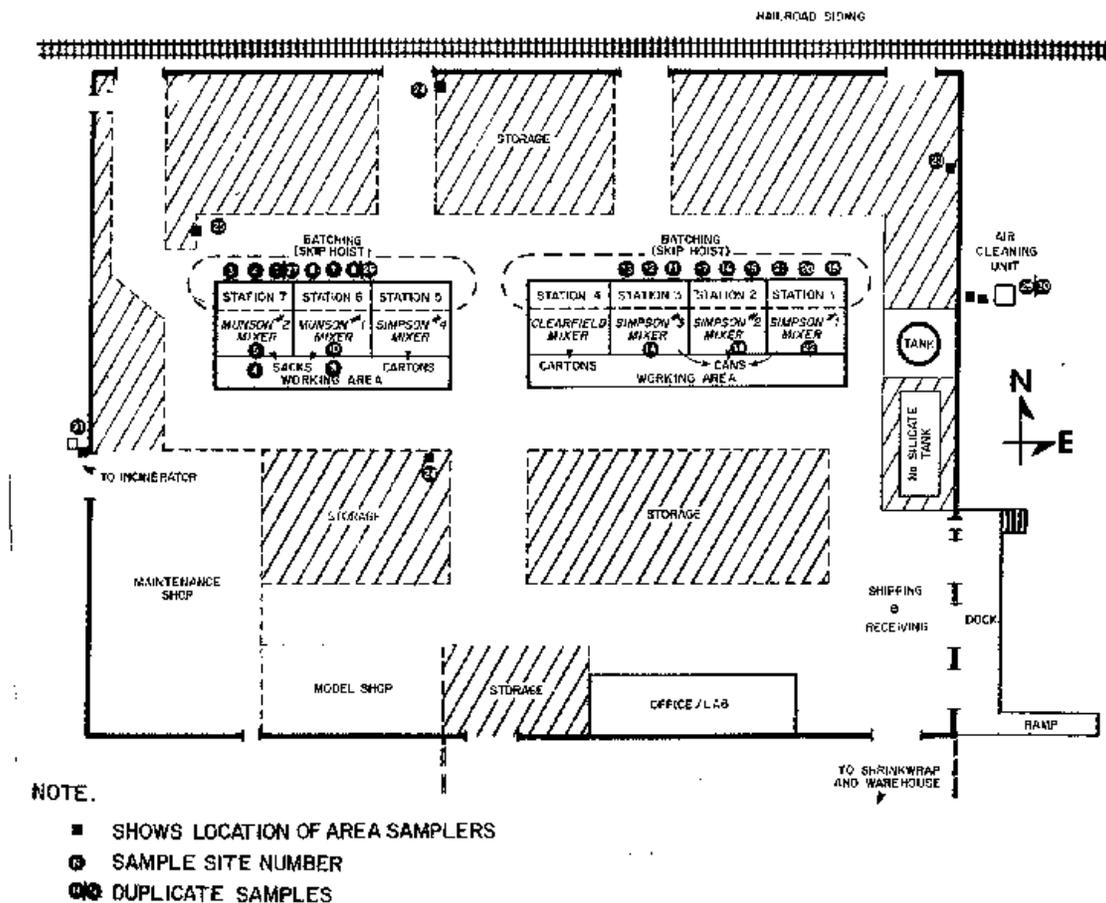
Figure 17. Plant layout showing area sampling sites
