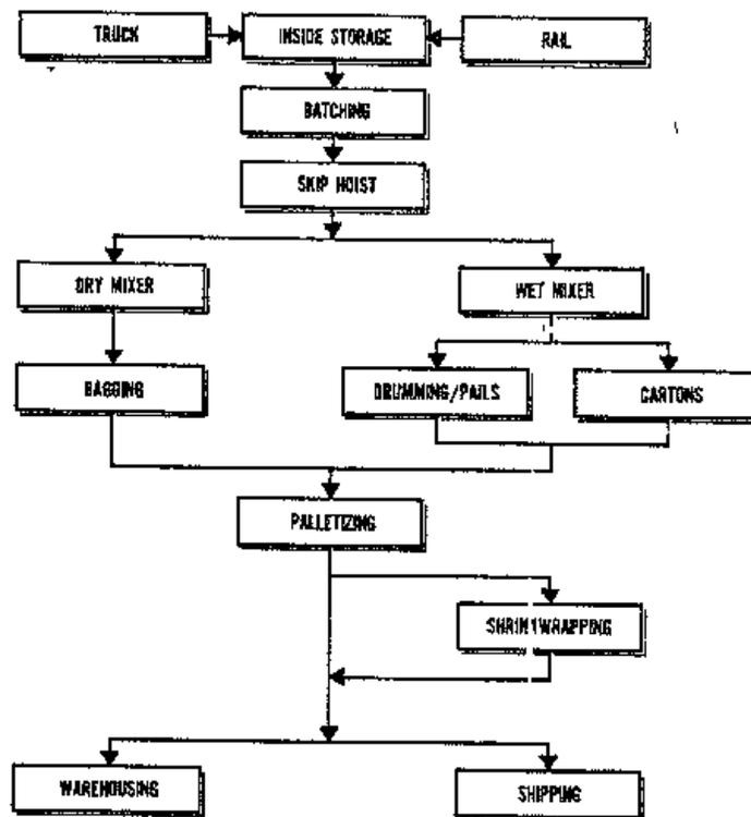
Figure 1. Process Flow Diagram
