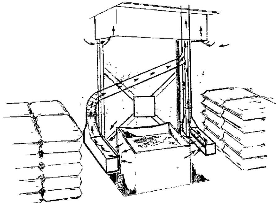
Figure 10. Typical batching station air flow
