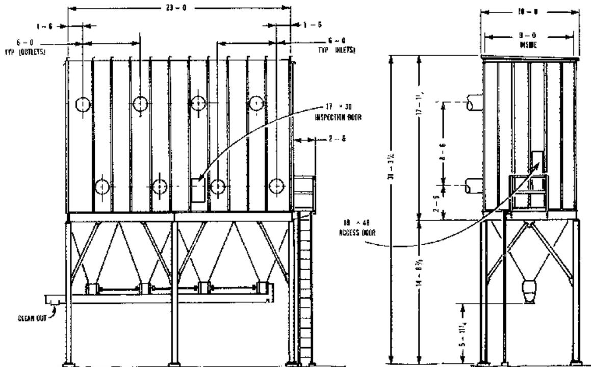
Figure 7. Dust collector details
