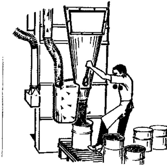
Figure 15. Typical pail filling station exhaust ventilation air flow
