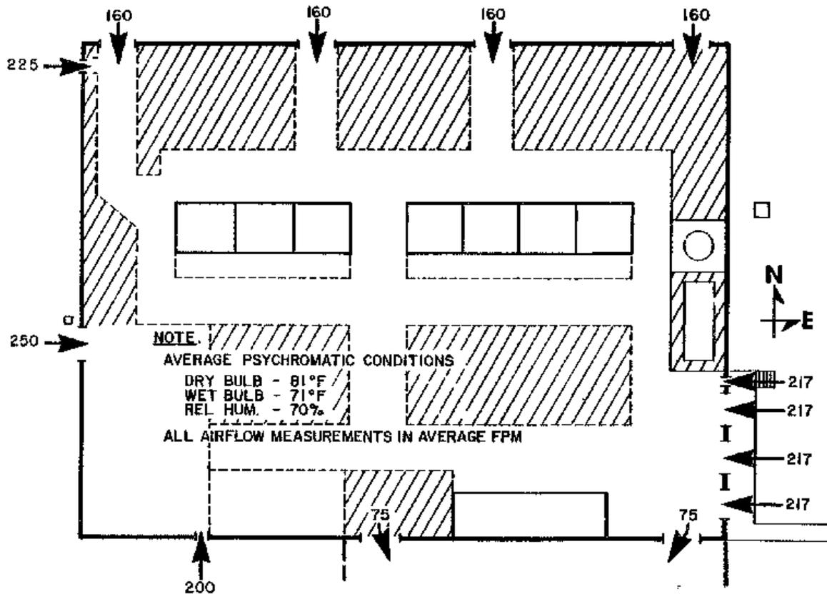
Figure 27. General ventilation through wall openings
