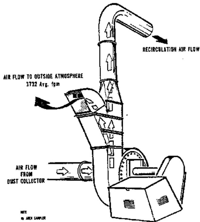
Figure 9. Dust collector blower air flow
