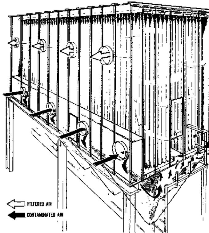
Figure 6. Dust collector air flow
