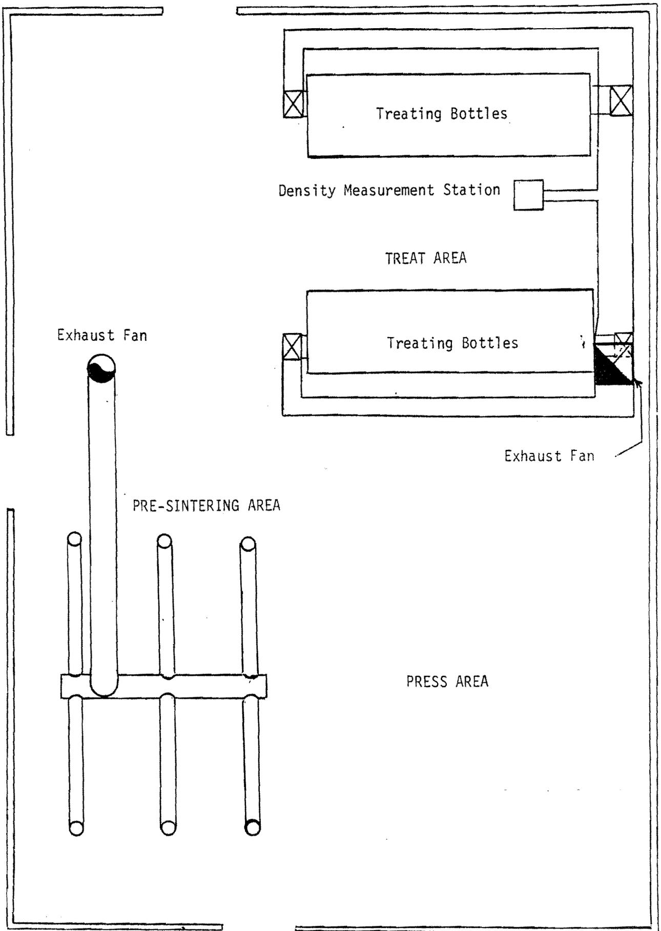
Figure 2. Press and Treat Room - Air Exhaust System.
