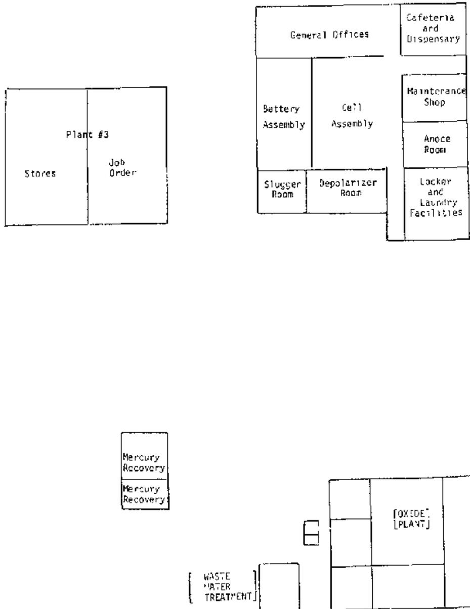
Figure 1. Layout Of The Battery Manufacturing Facility
