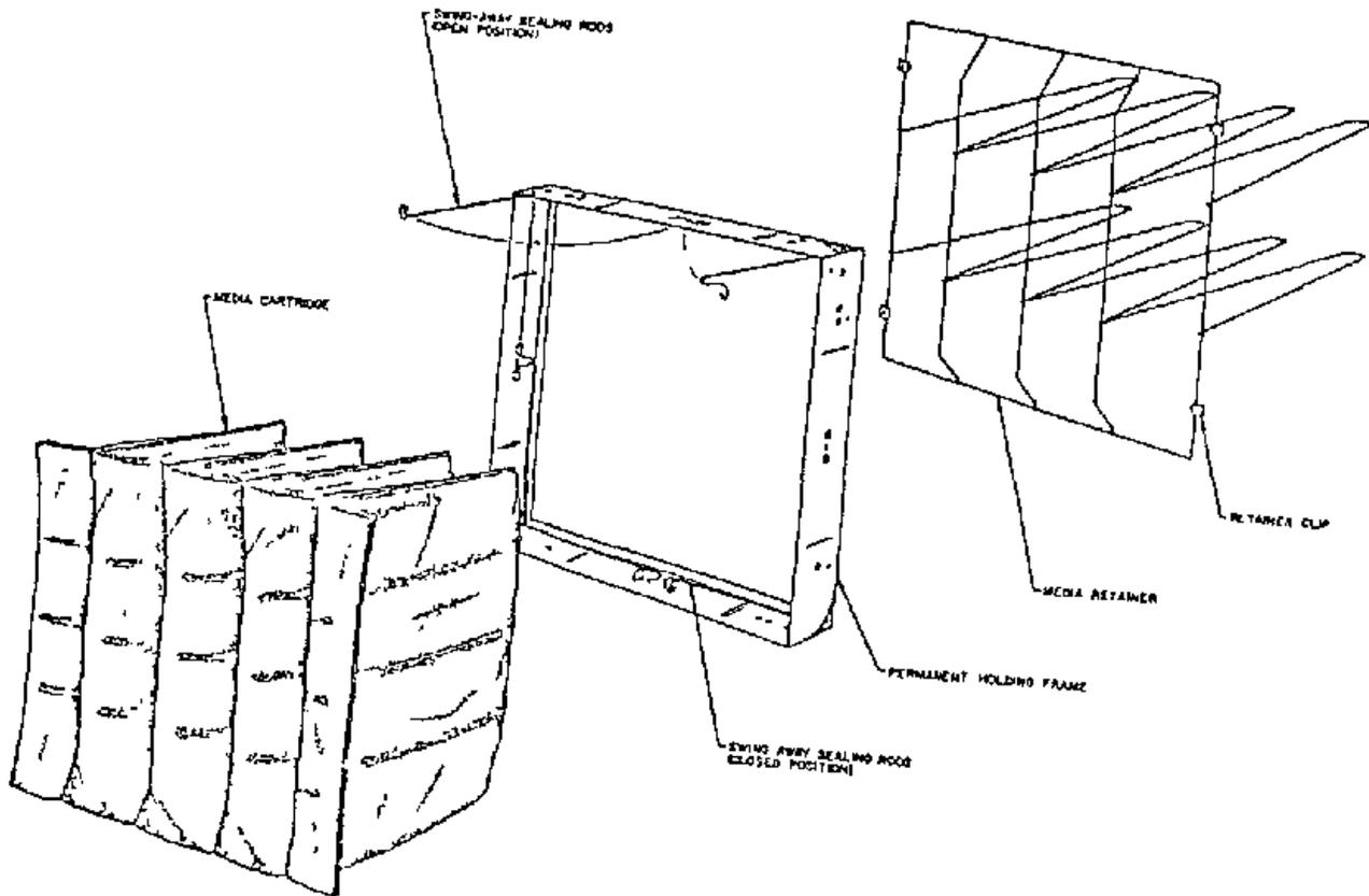
Figure 16. Fiber Filters for Particulate Removal.
