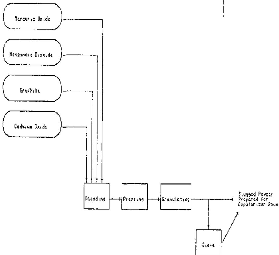
Figure 3. Slugger Room - Process Flow Diagram
