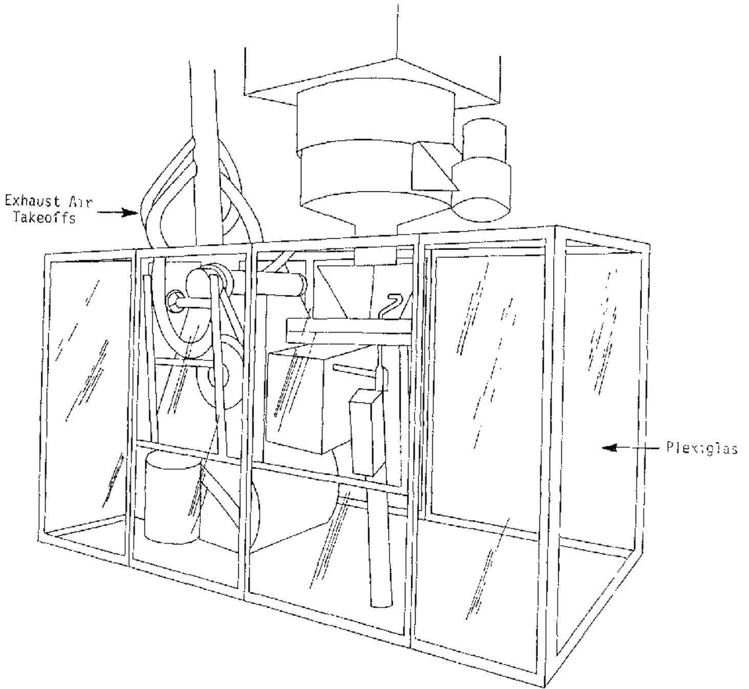
Figure 9 Plexiglas Machine Enclosure
