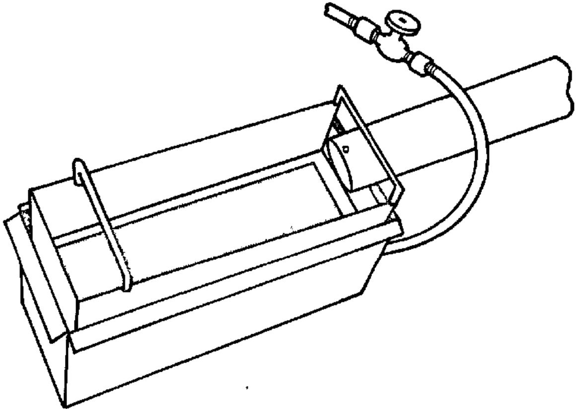
Figure V-4. Exhaust Tube Tip Container.
