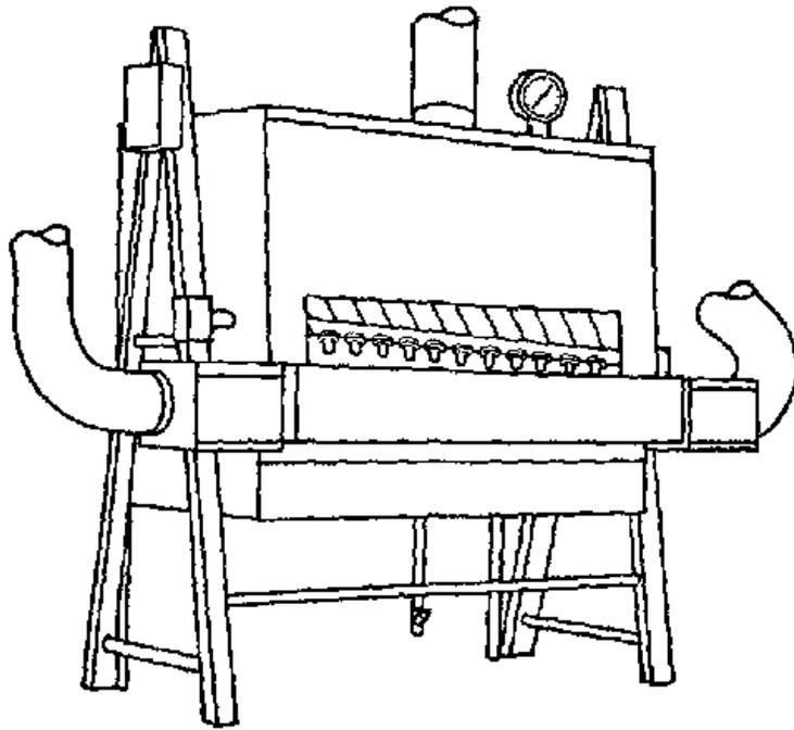
Figure V-12. Mercury Fill Station Hood.
