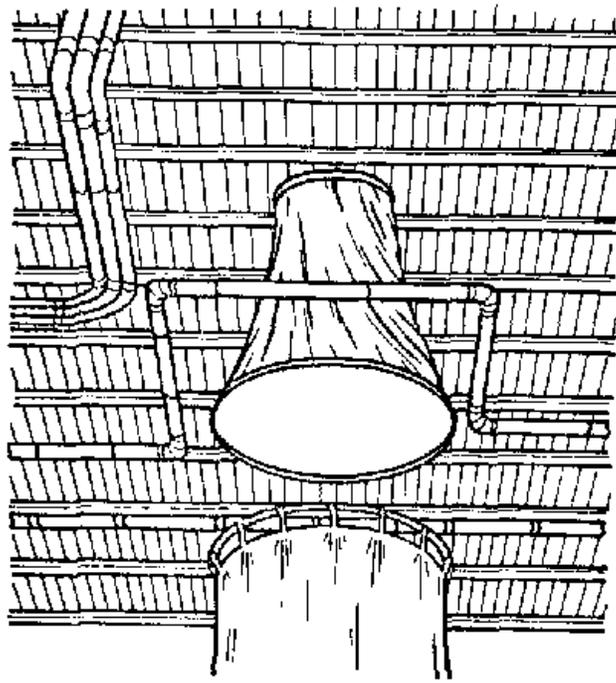
Figure V-15. Shroud Over Exhaust Machine.
