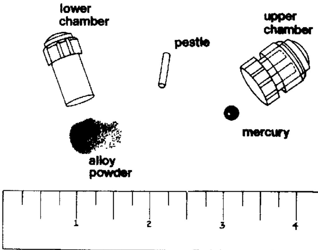
Figure V-2. Dispersalloy<sup>R</sup> Dispos-a-cap Component.
