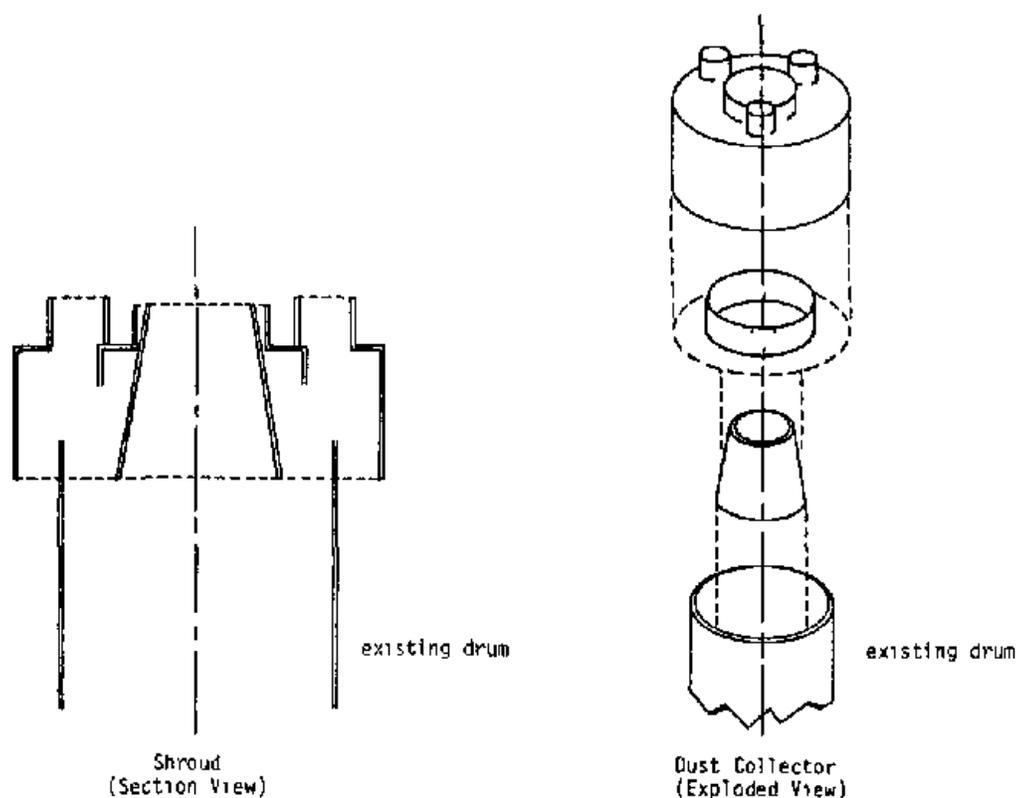
Figure V-19. Schematic Drawing of Drum Loading Hood.
