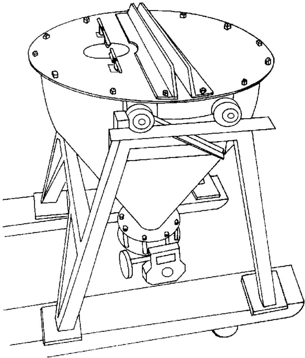
Figure V-7. Material Transfer Container (Pod).
