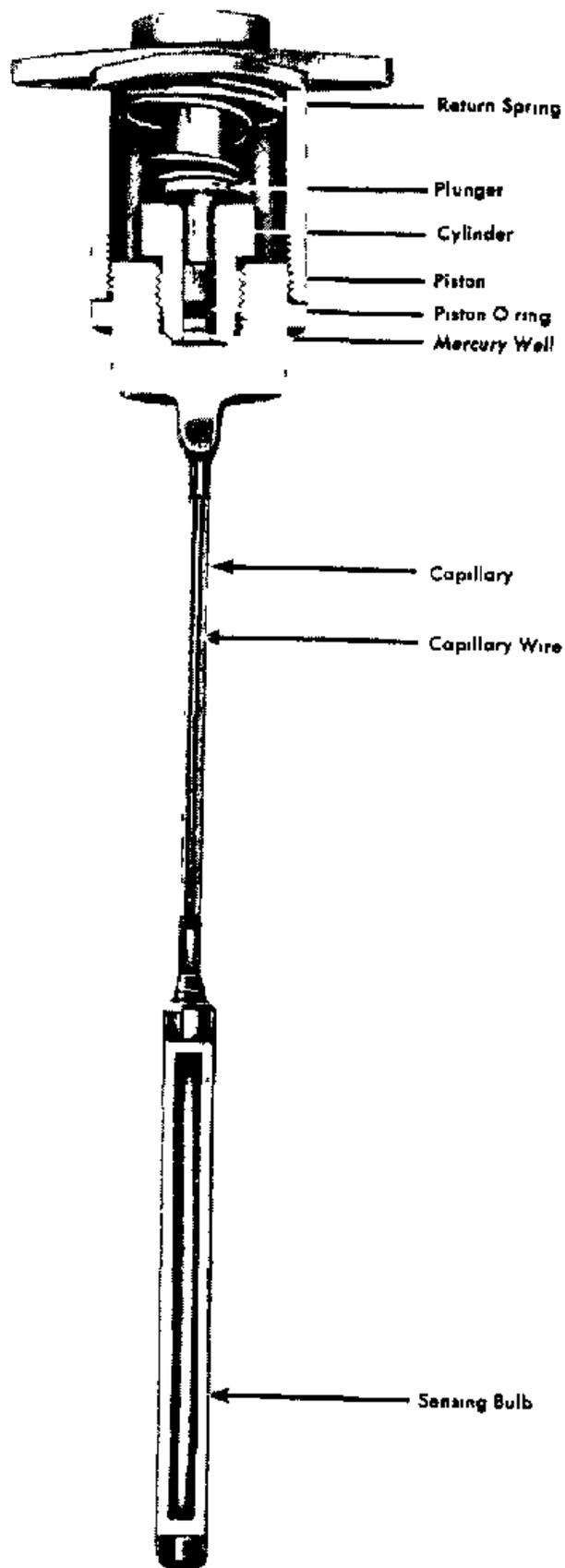
Figure IV-1. Temperature-Sensing Instrument.
