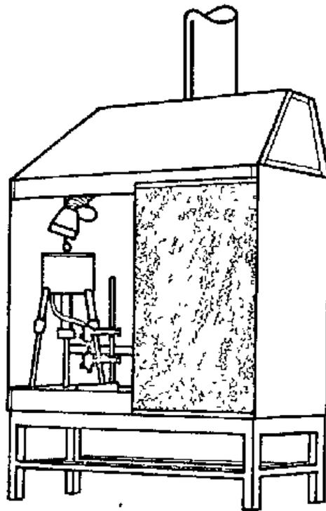
Figure V-14. Mylar Sheet Across the Face of the Exhaust Hood.
