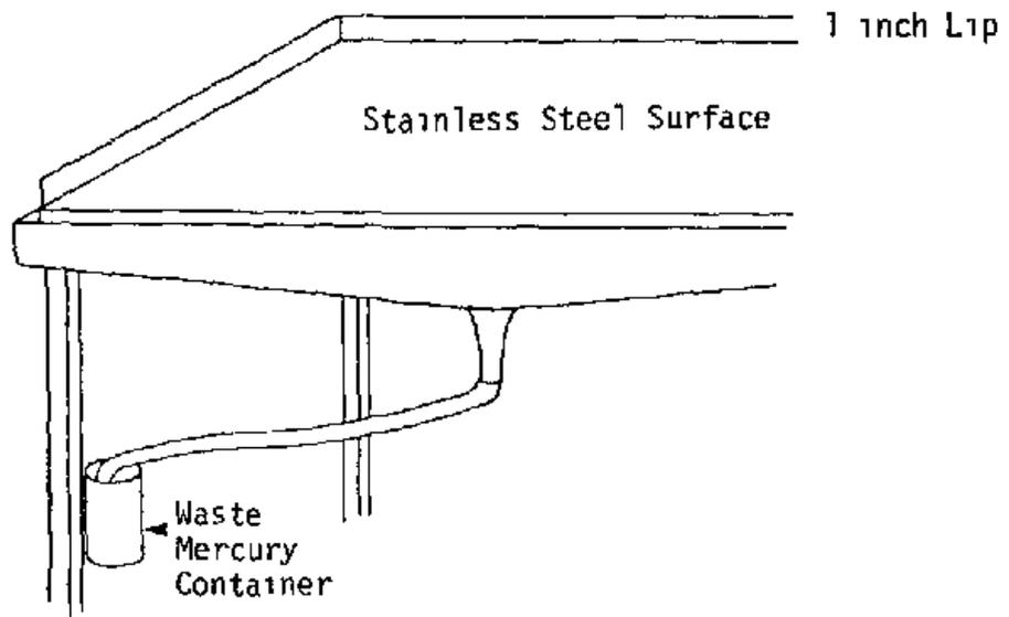
Figure VI-1 Work Station with Drainage Trough
