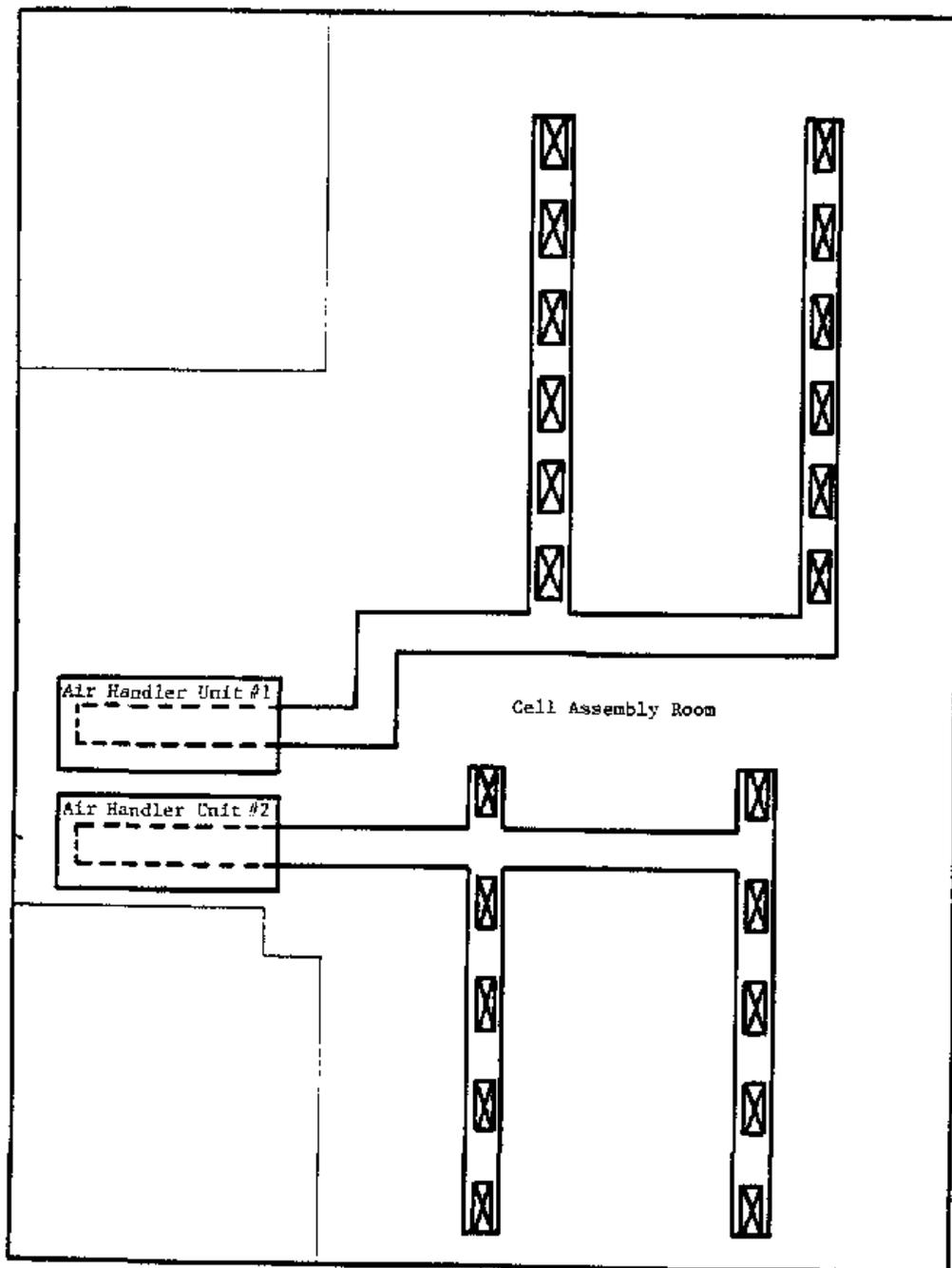
Figure V-23. Schematic of Recirculating Air System.
