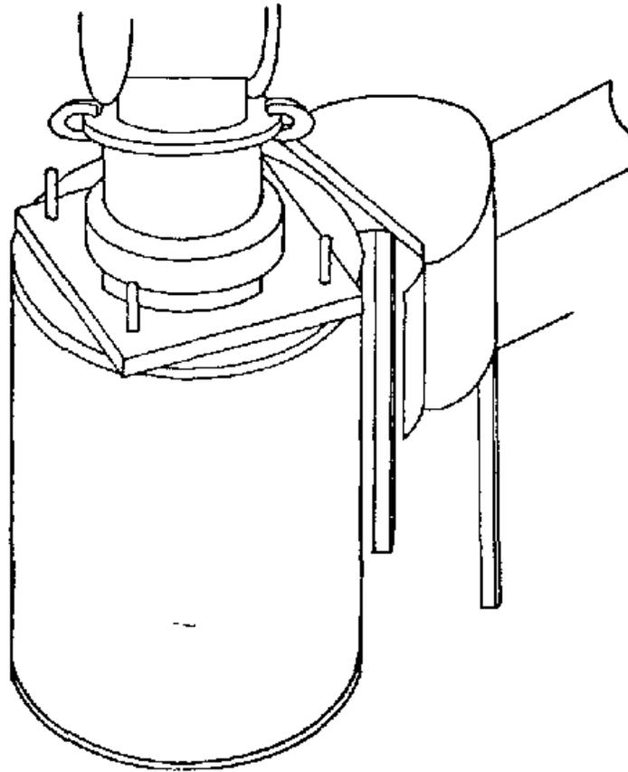
Figure V-16. Exhaust Air Takeoff at Drum Loading Stand.
