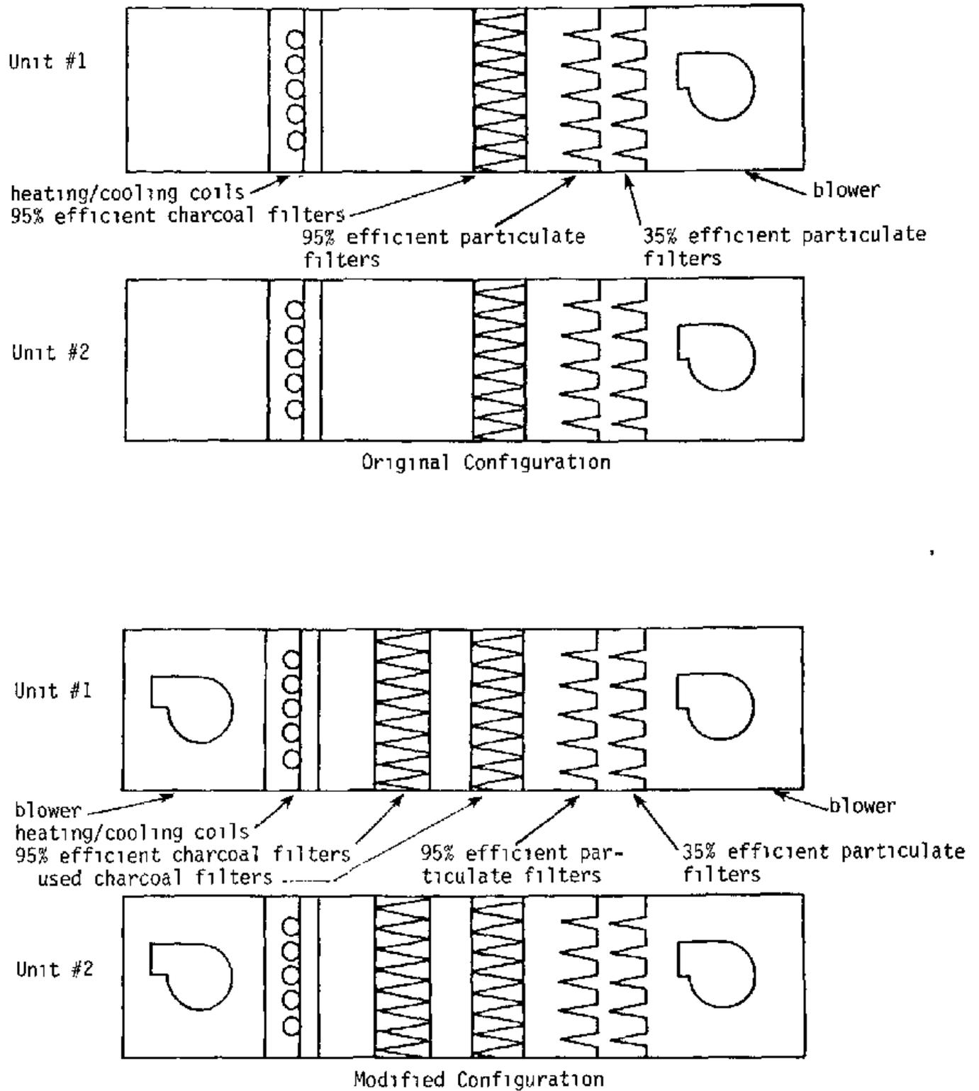
Figure V-25. Original and Modified Air Handler Configurations.
