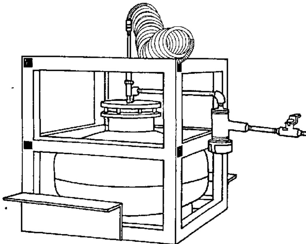
Figure V-6. Mercury Storage Container.
