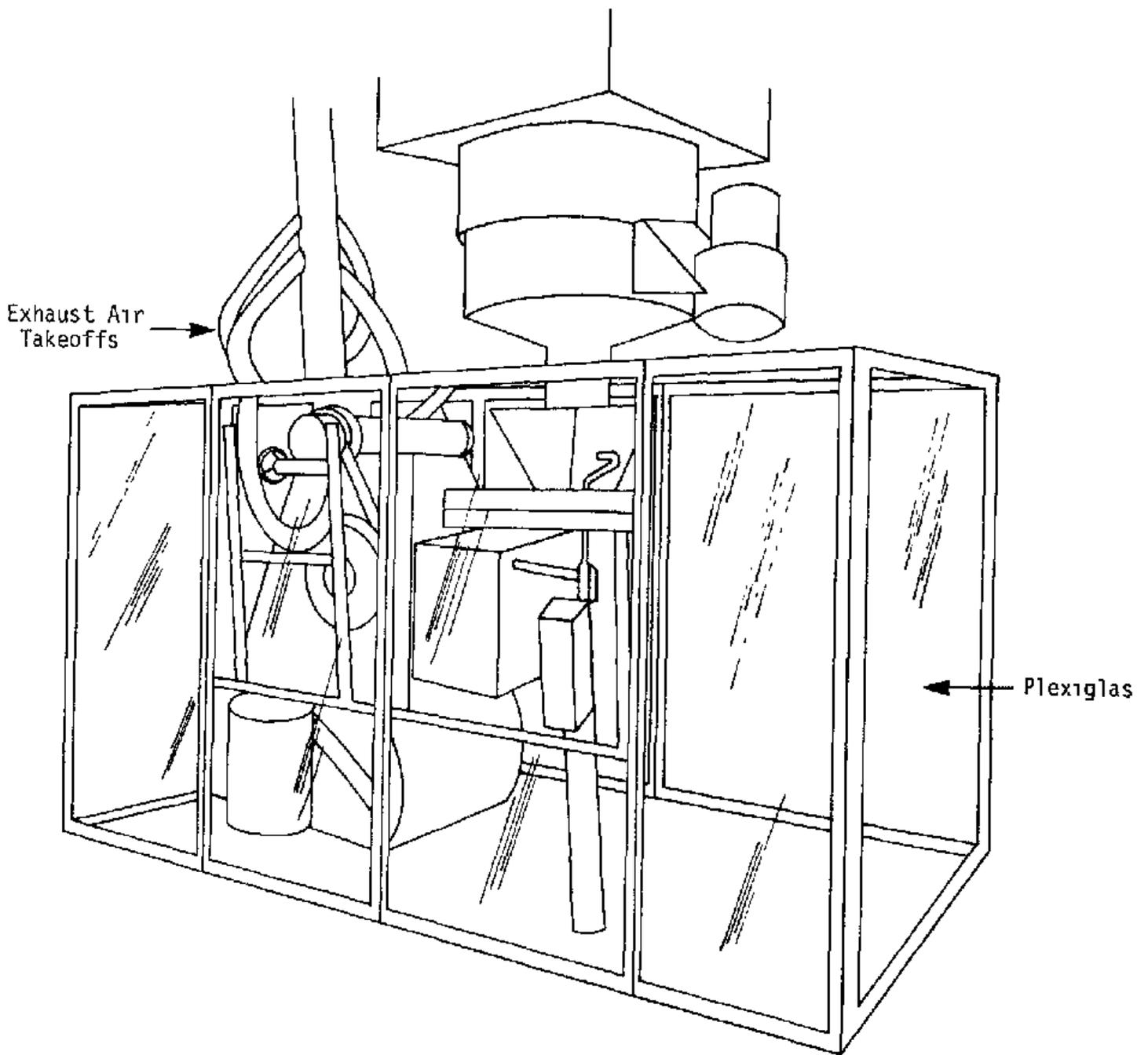
Figure V-10. Plexiglas Machine Enclosure.
