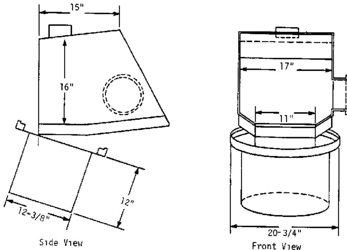
Figure V-18. Mercuric Oxide Charger Hood Design.
