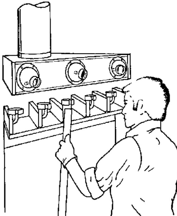
Figure V-21. Adjustable 2-Inch Supply Air Vents.
