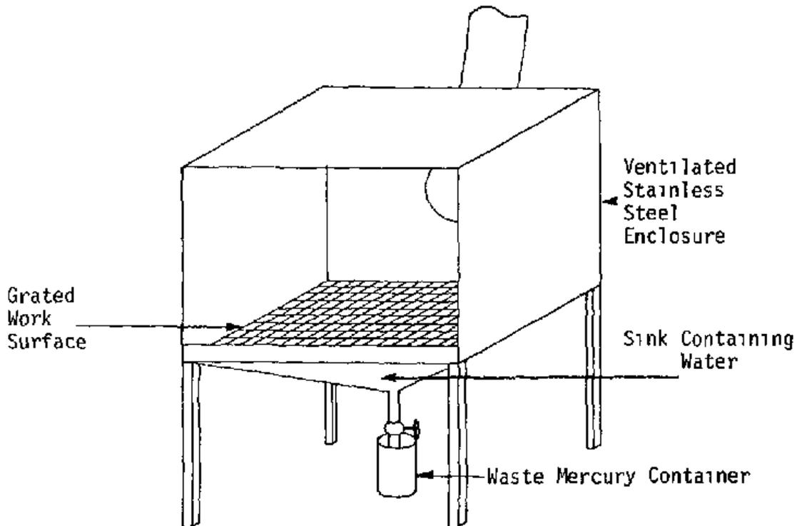
Figure VI-2. Ventilated Work Station with Grated Surface
