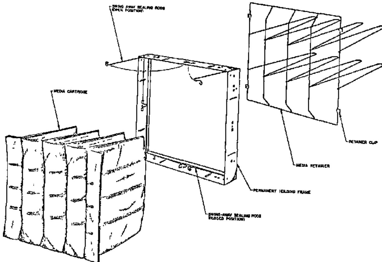
Figure V-24. Fiber Filters for Particulate Removal.
