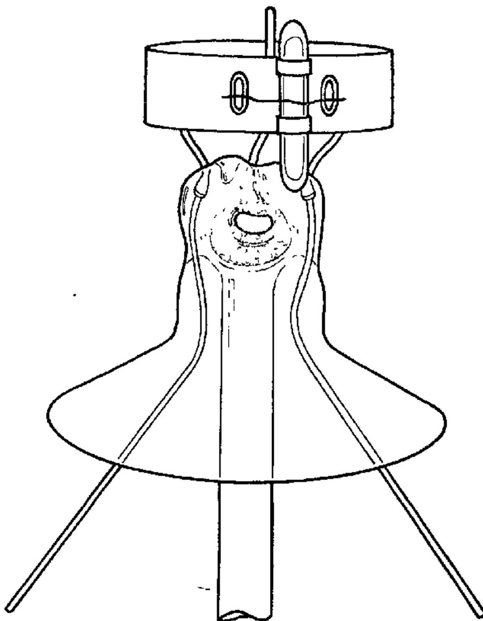
Figure V-3. Mount Assembly with Mercury P111.
