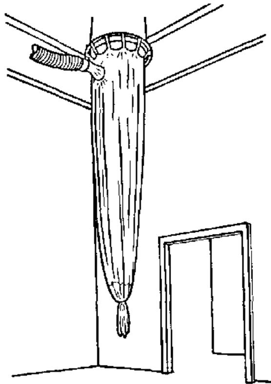
Figure V-17. Filter Bag for Removing PMA from Exhaust Air.
