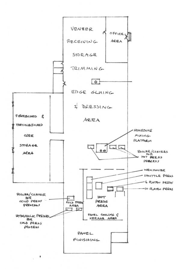
FIGURE 1. DIAGRAM OF HILLCREST UBNEER PLANT
