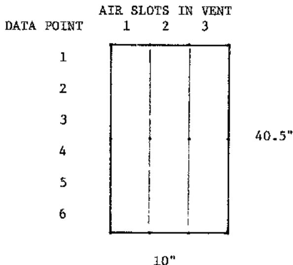
Note: The width of the vertical air slots varies from 3.25" to 4" and results in different data point areas.
