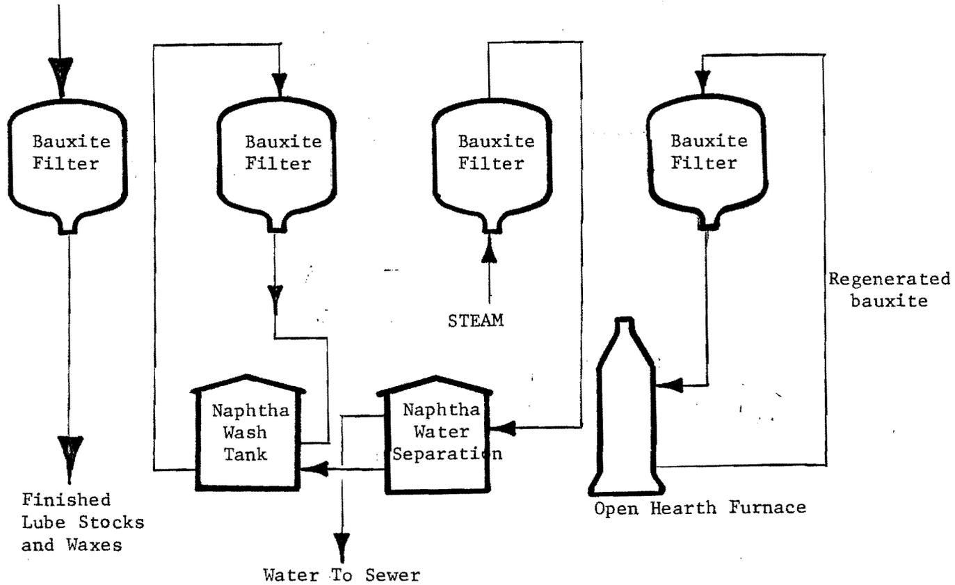
FIGURE 3-3 BAUXITE FILTERS
