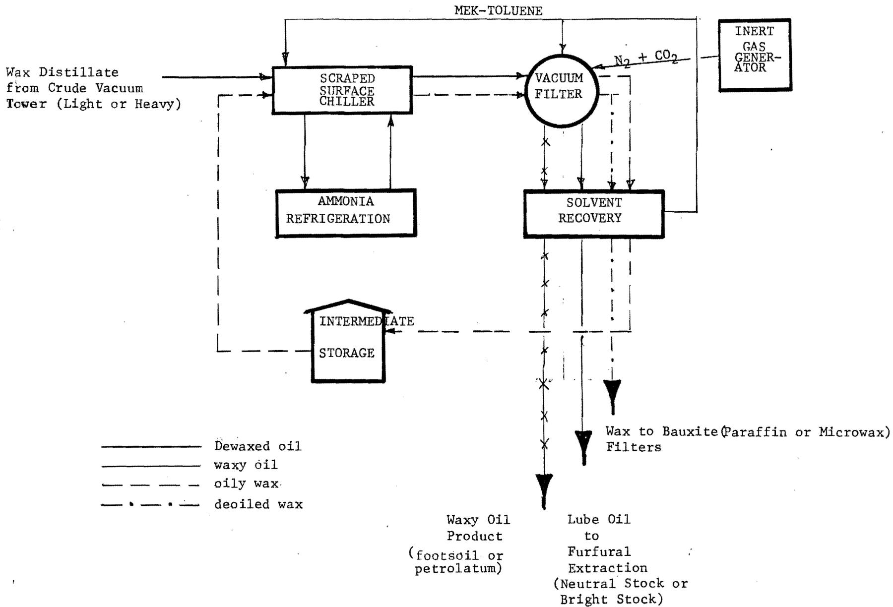
The deoiled wax from the filter drum is steam stripped for solvent recovery and goes to the bauxite clay filter for final treatment before sale. Wax product from the light wax distillate is called paraffin wax and wax product from the heavy wax distillate and DRO is called microwax.
