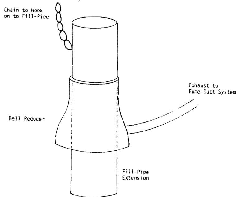
Figure 4. Fill-Pipe Extension
