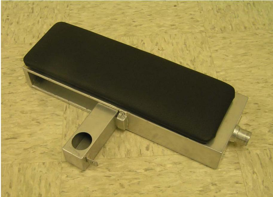
Figure 10: Hand rest exhaust
