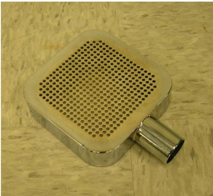
Figure 9: Rectangular side exhaust hood
