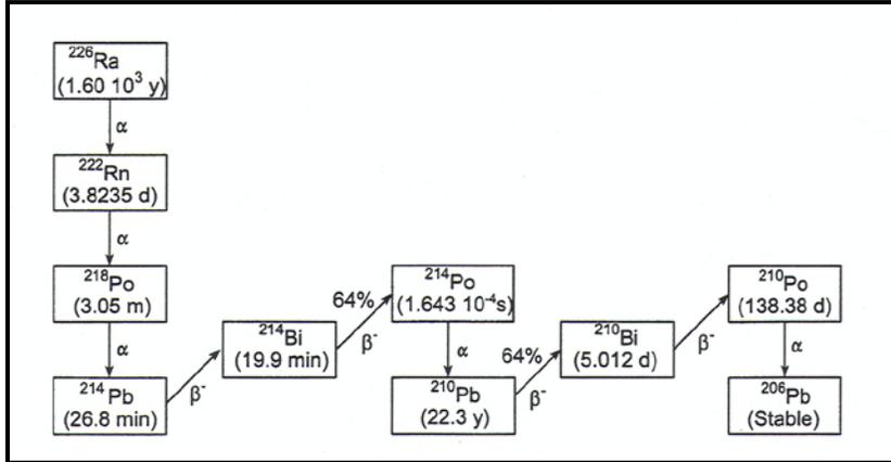
Figure 1. Ra-226 decay series (from ICRP 1998).
