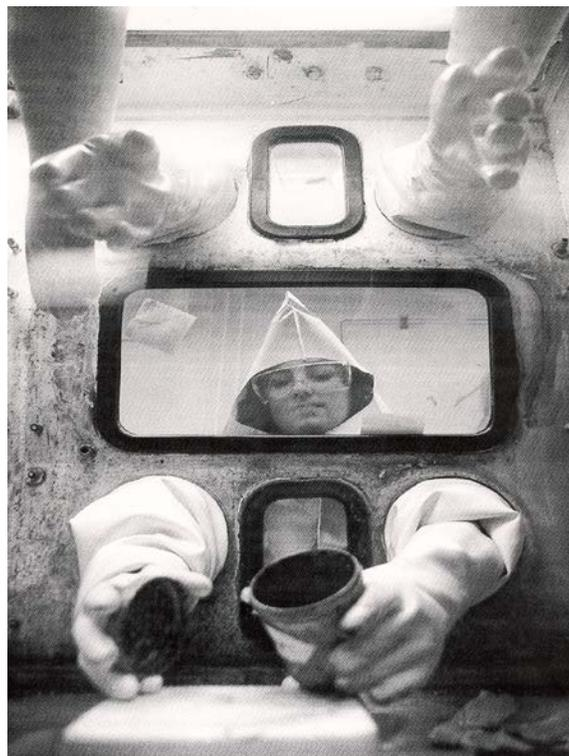
Figure 5 Other plutonium gloveboxes at Hanford. Note the viewing area in direct line with the lower torso in the center between the gloves.<sup>(2)</sup>
