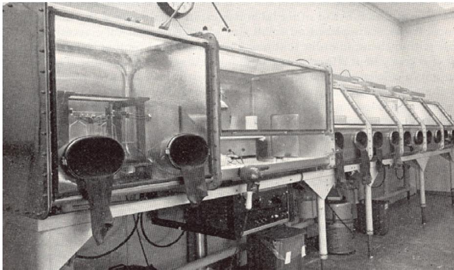
Figure 4 Plutonium gloveboxes at LANL's CMR facility<sup>(1)</sup>
