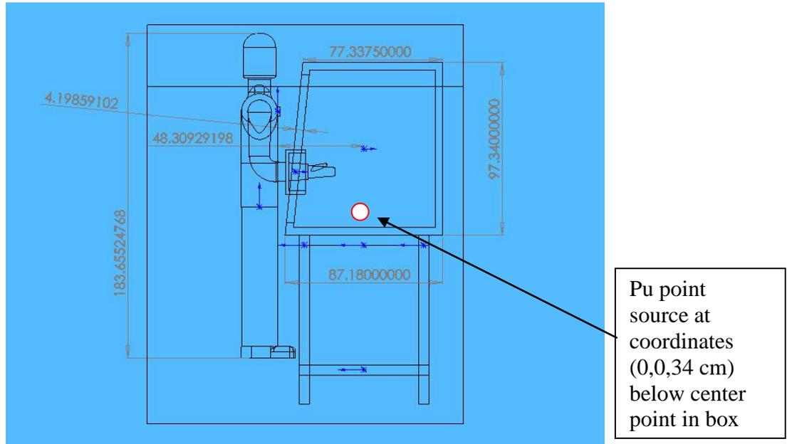
Figure A1 Dimensions (all lengths are in centimeters)
