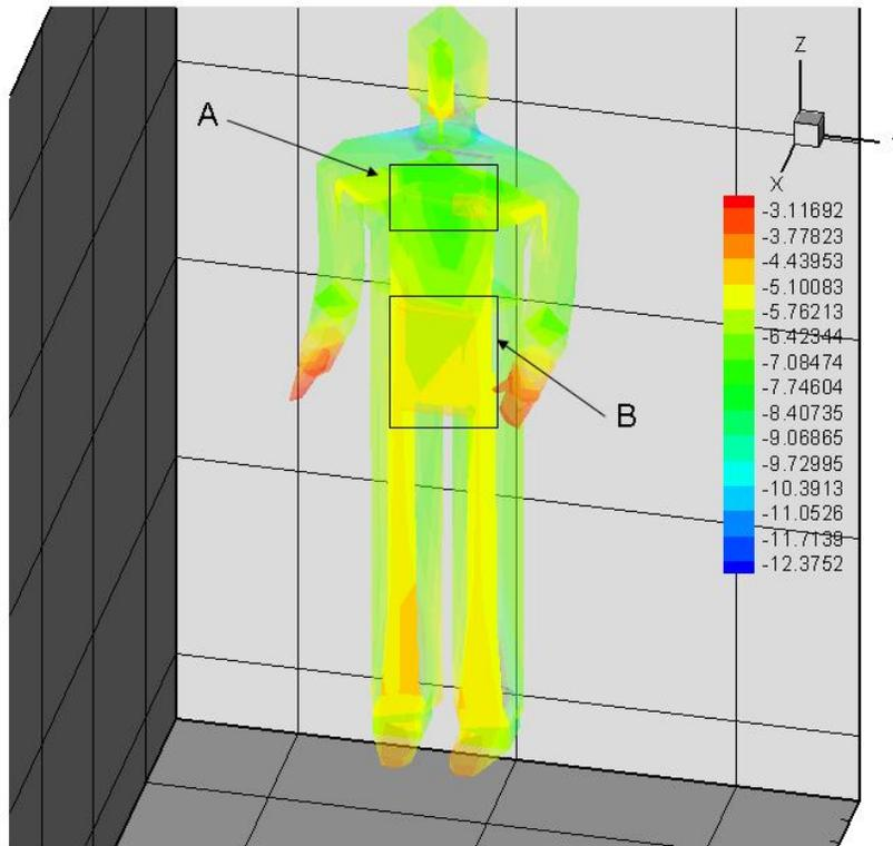
Figure 8 Data point selection regions. Various colors signify relative magnitude of flux across a selected plane on the x-axis.
