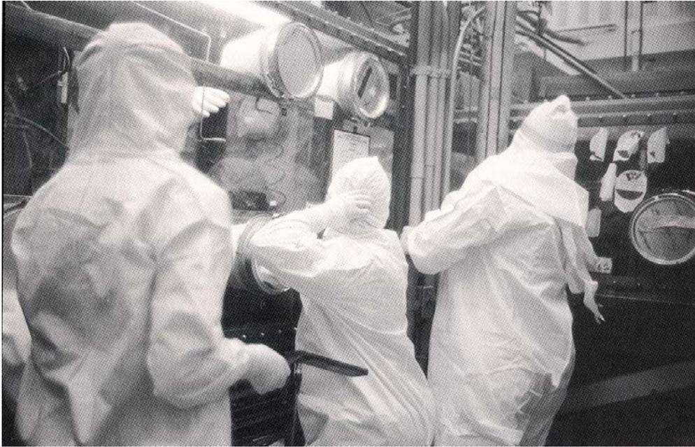
Figure 3 Plutonium gloveboxes at Hanford<sup>(2)</sup>
