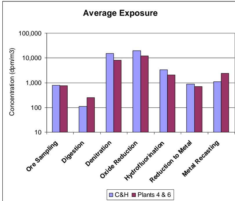
**Figure 4. Comparison of C&H Tabulated Average Exposure with Mallinckrodt Plants 4 and 6 Average Exposure**
