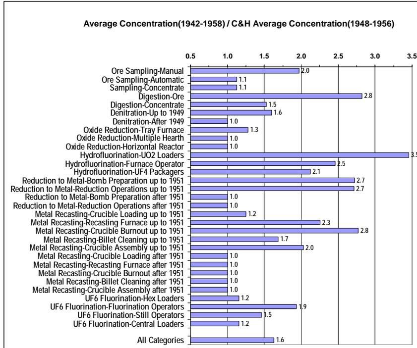
**Figure 8. Comparison of Estimated Average Exposure (dpm/m<sup>3</sup>) from 1942 to 1958 with C&H 1948 to 1956 Average Exposure (dpm/m<sup>3</sup>) (Assumes 95<sup>th</sup> Percentile Estimate for Years 1942 to 1947)**
