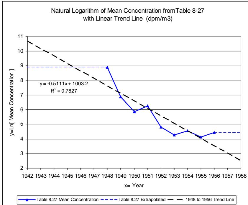
**Figure 10. TBD-6001 Table 8.27 Mean Air Concentrations from 1948 to 1956, with Extrapolation to Earlier and Later Years and Regression Trend Line (n=9, R<sup>2</sup>=0.78)**
