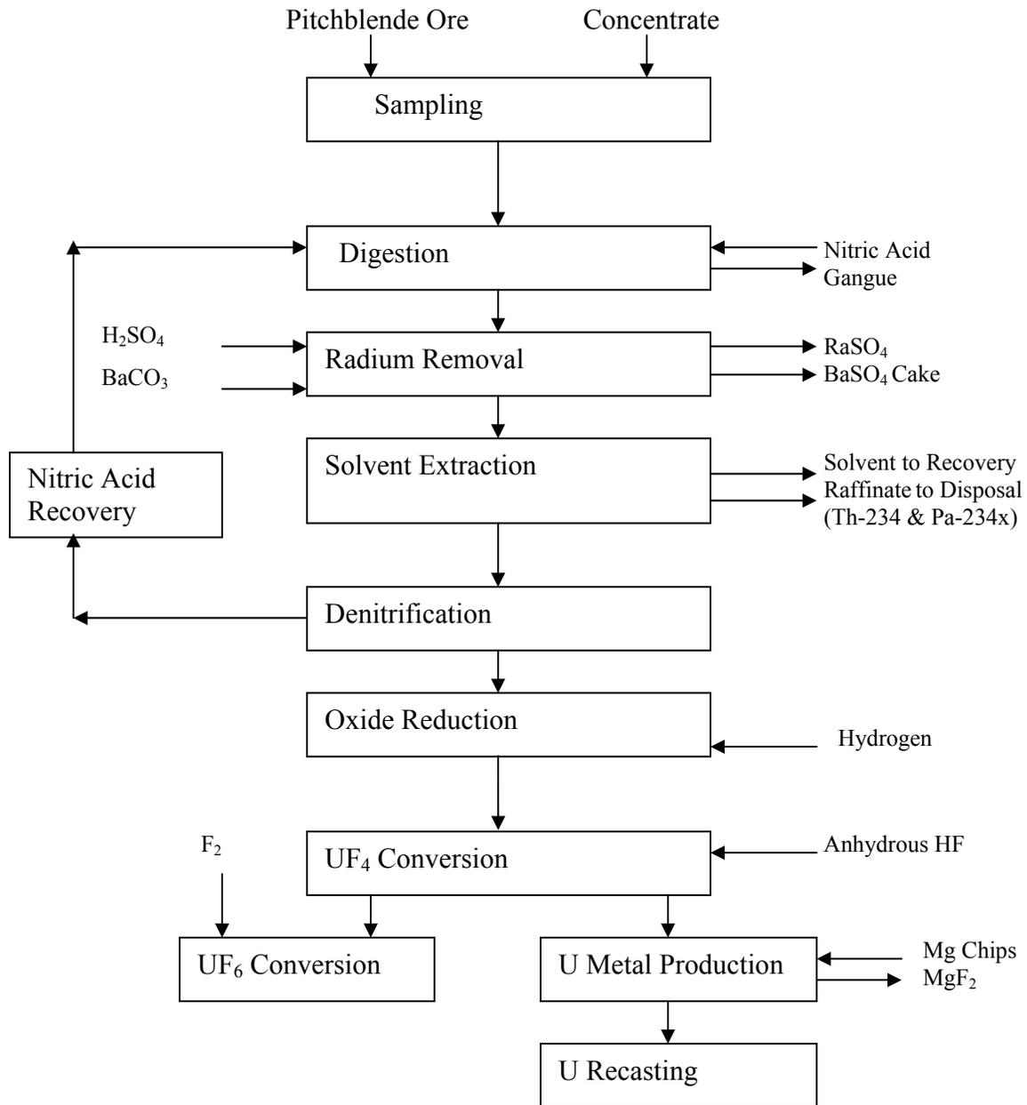
**Figure 1. Flow Diagram for Uranium Refining from Ore or Concentrates**
