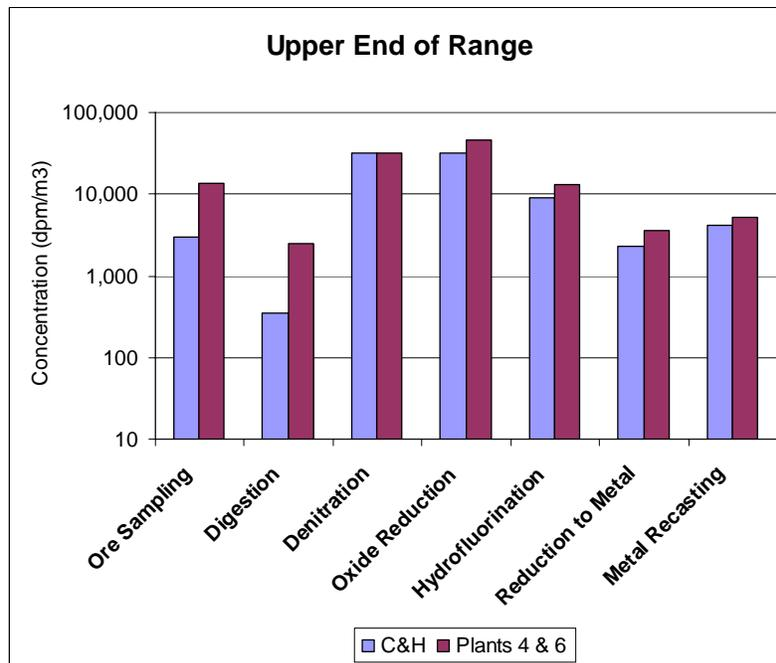
Figure 3. Comparison of C&H Tabulated Upper End of Range with Mallinckrodt Plants 4 and 6 Upper End of Range
