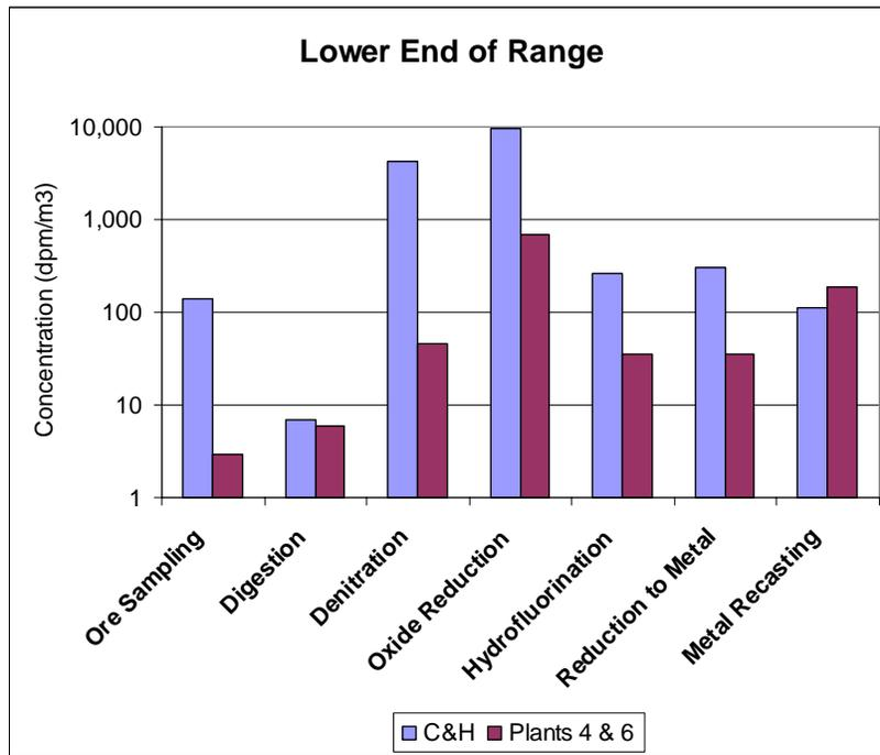
Figure 2. Comparison of C&H Tabulated Lower End of Range with Mallinckrodt Plants 4 and 6 Lower End of Range
