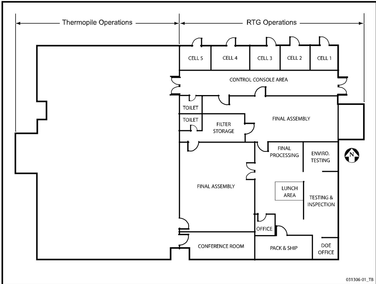
Figure 2-11. Layout of Building 400 (GE 1982b, pg. 9).
