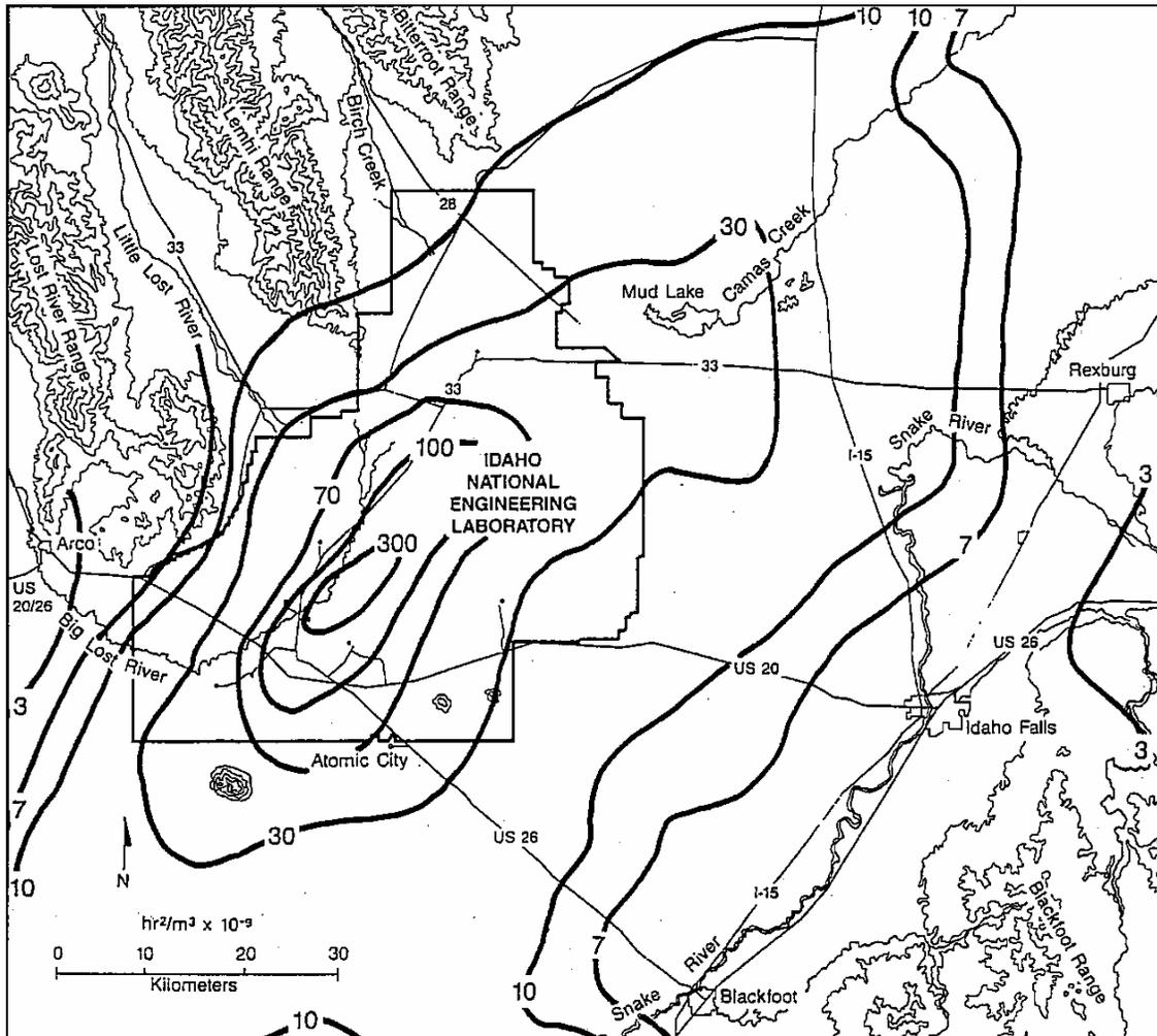
Figure 4-3. Nine-year (1974 to 1983 excluding 1978) average mesoscale dispersion isopleths of air concentration at ground level ( $\text{hr}^2/\text{m}^3 \times 10^{-9}$ ), normalized to unit release rate (DOE 1991).
