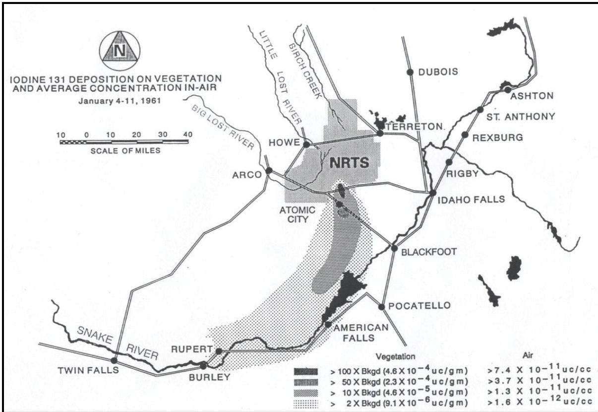
Figure 4-6. Dispersion coefficient contours for the SL-1 accident (redrafted from Horan and Gammill 1961).
