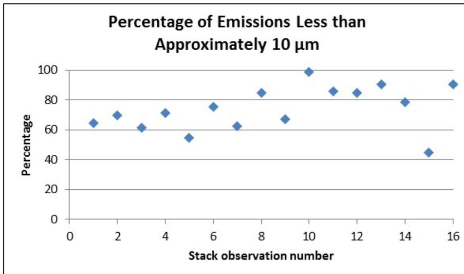
Figure 4-3. Percentage of stack emission less than approximately 10 μm AMAD (Spenceley 1985).
