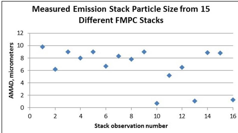
Figure 4-2. Measured emission stack particle size from 15 different FMPC stacks (Spenceley 1985).
