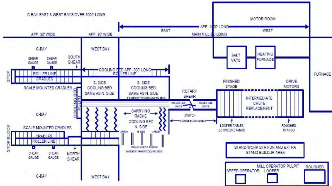
FIGURE 3-1. BETHLEHEM STEEL 10-INCH BAR MILL LINE DIAGRAM
