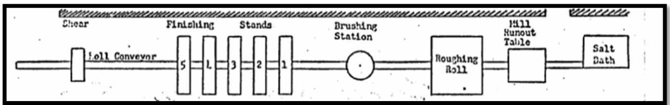
Figure 5-2: Layout of Hot Strip Uranium Mill Operation at Superior Steel Co., 1955 (Myrick, 1981)
