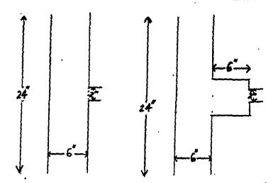
The 2" pipe leading away from the column does not tie directly into the 2h" section but rather into the 6" tee on the side of the section.
