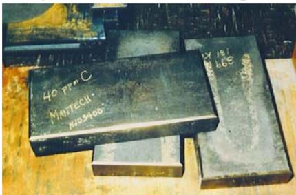
USAF Mantech castings – unalloyed DU for sheet rolling to reproduce Oak Ridge Y-12 material produced for LANL.
