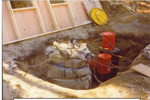
Crude outdoor drum heating test stand. 55 gallon drum inside 85 gallon drum filled with anti-freeze. Insulated to reduce heat loss.
