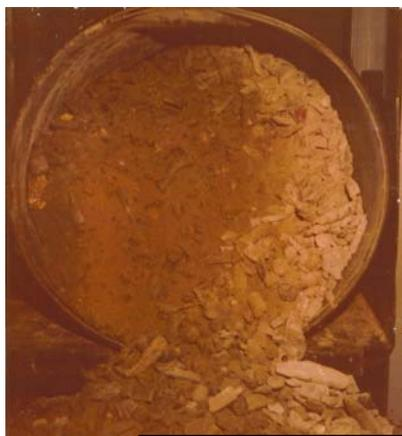
Initial inspection of 55 gallon drum scrap. Waste composed of sand, uranium bullet fragments and aluminum sabots.
