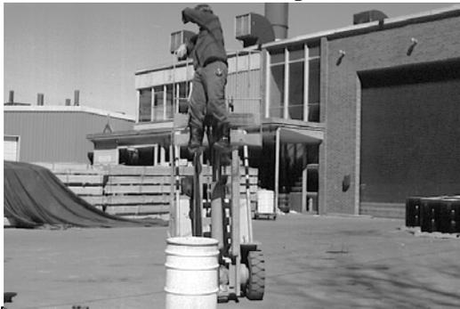
Employee performing crude DoT impact penetration test behind Building C to test for foam barrel puncture resistance.
