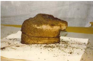
Briquetted DU machine turnings removed from foundry crucible. DU metal trapped in oxide layers could not be reclaimed. Note DU oxide powder everywhere in work area.
