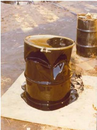
Prior to switching to anti-freeze, heated quench oil was used to heat the test drums. This test drum was removed after testing and is coated in oil. The drum collapsed from a vacuum produced by oxidizing uranium chips that scavenged available oxygen inside the drum.
