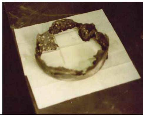
removed foundry crucible residue of unmelted Niobium pellets and uranium. Higher temperatures were required, necessitating the development of better mold wash coatings. Alternative VIM process to Rocky Flats eb melting trials.
