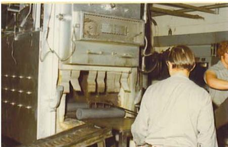
Unloading extrusion billets. No work gloves, no safety glasses.
