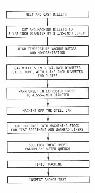
Figure 1. General Process Flow Chart for DU-6.5Nb, DU-8Mo and DU-3/4Ti Alloys
