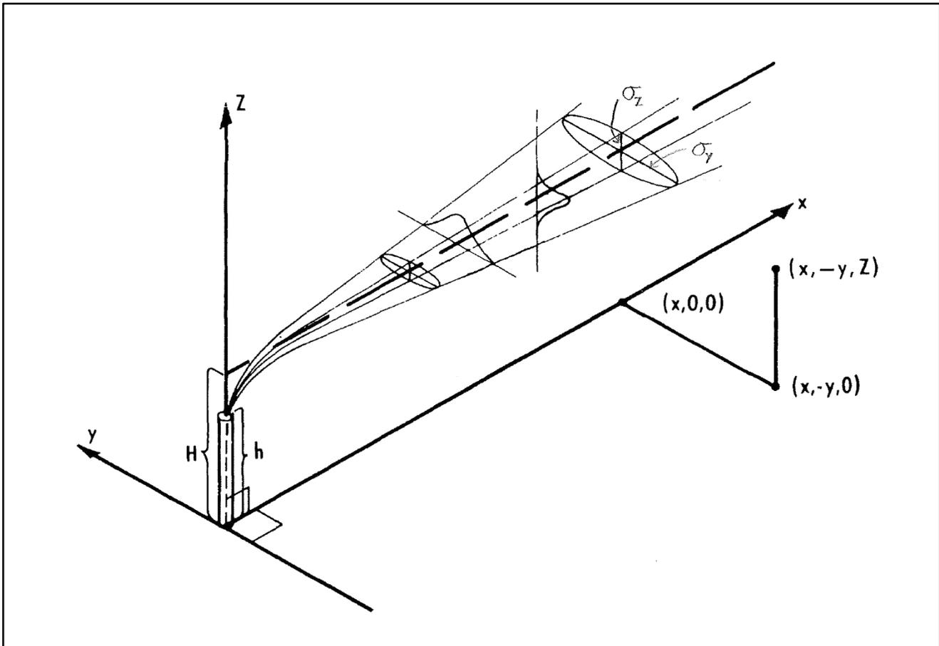
Figure 5-2. Illustration of Gaussian plume model (Turner 1970).
