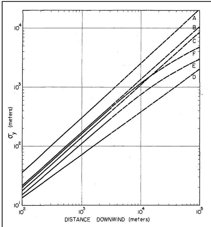
Figure 5-3. Horizontal atmospheric dispersion coefficients (Yanskey, Markee, and Richter 1966).
