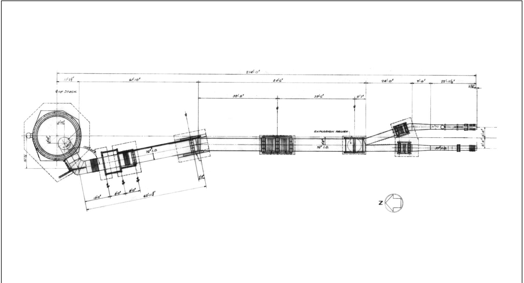
Figure 3-4. IET Facility exhaust system during IET #10 runs (Parsons 1963).
