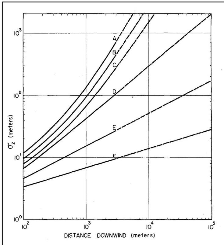
Figure 5-4. Vertical atmospheric dispersion coefficients (Yanskey, Markee, and Richter 1966).
