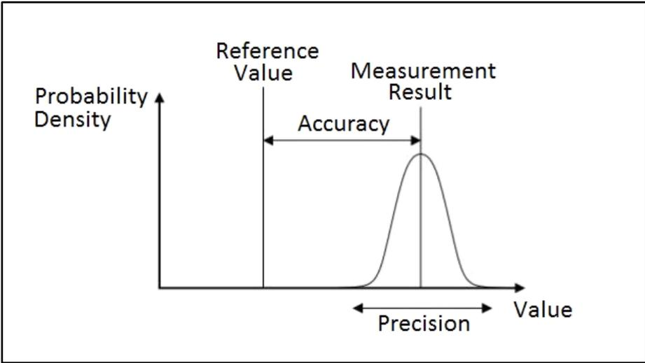
Figure 8-1. Relationship of measurement accuracy and precision to the reference value.
