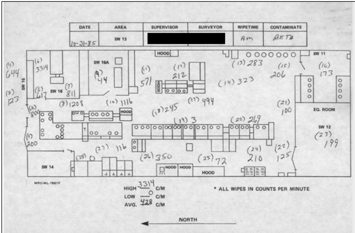
Figure 3. Typical contamination swipe locations in Room SW-13.
