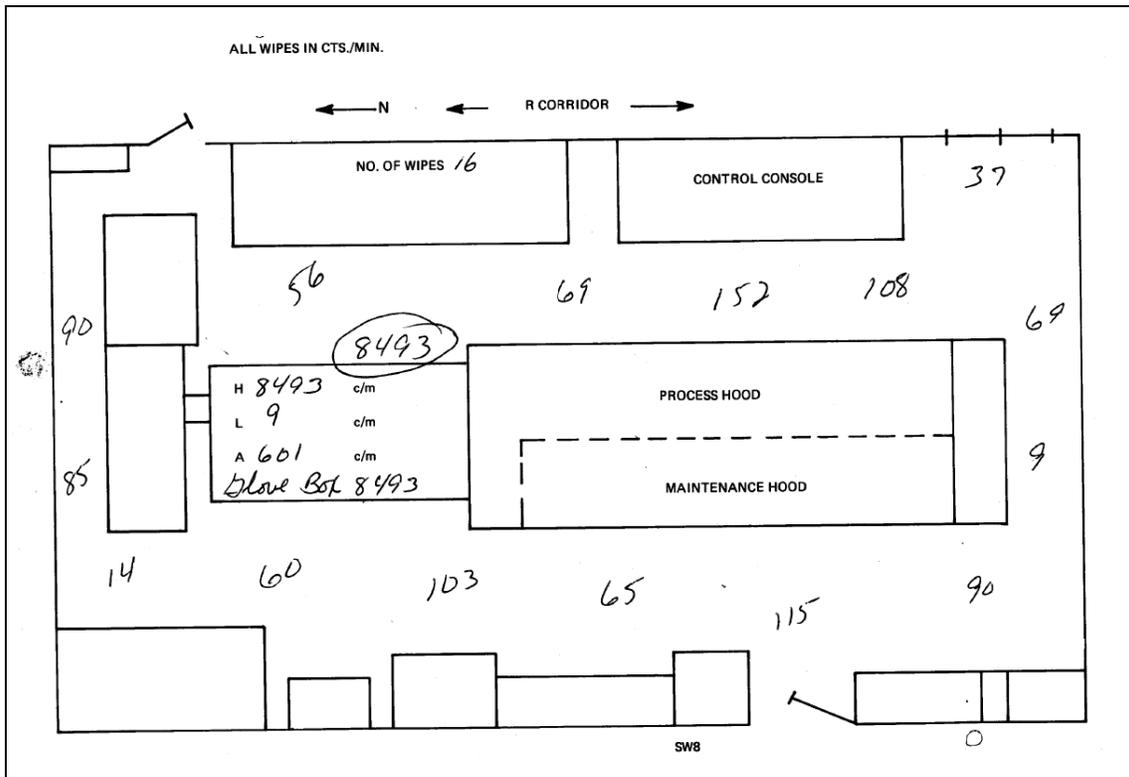
Figure 4. Typical contamination swipe locations in Room R-108.
