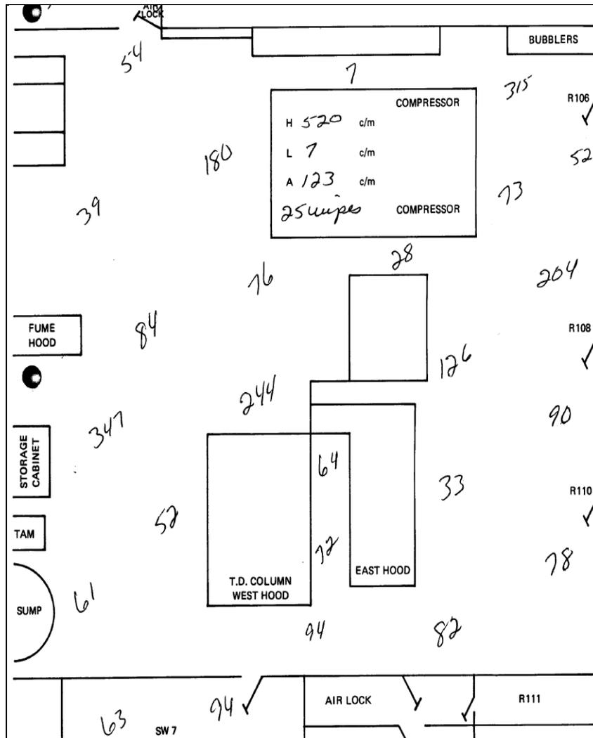
Figure 5. Typical contamination swipe locations in Room SW-8.
