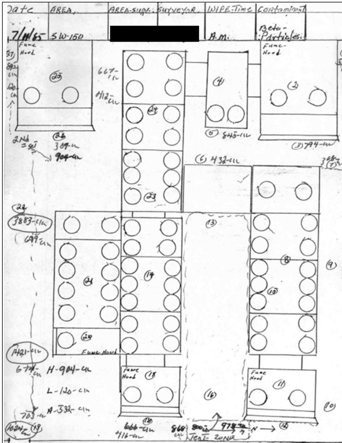
Figure 2. Typical contamination swipe locations in Room SW-150.
