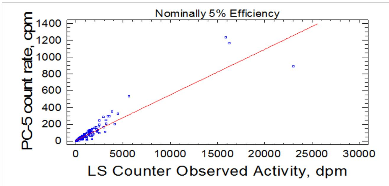
Figure 11. Calibration of PC-5 based on paired LSC counts.
