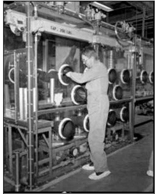
Figure 10. Worker at thorium glovebox containment. Source: Coughenour (2009). The photograph is unclassified and does not contain UCNI.
