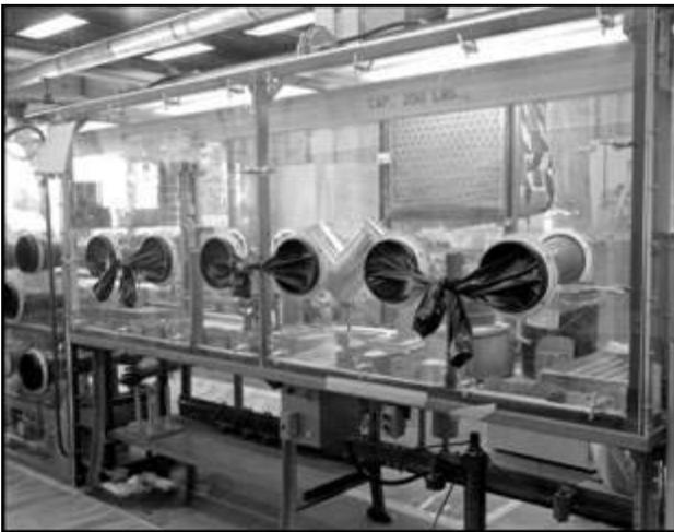
Figure 7. Thorium glovebox during operations. Note the thorium slugs lying horizontal in the far right of the glovebox. Source: Coughenour (2009). The photograph is unclassified and does not contain UCNI.
