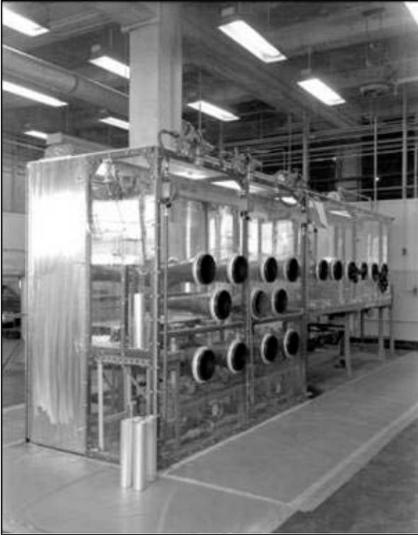
Figure 5. Thorium glovebox during construction. Note the highbay setting and partial height walls. Source: Coughenour (2009). The photograph is unclassified and does not contain UCNI.
