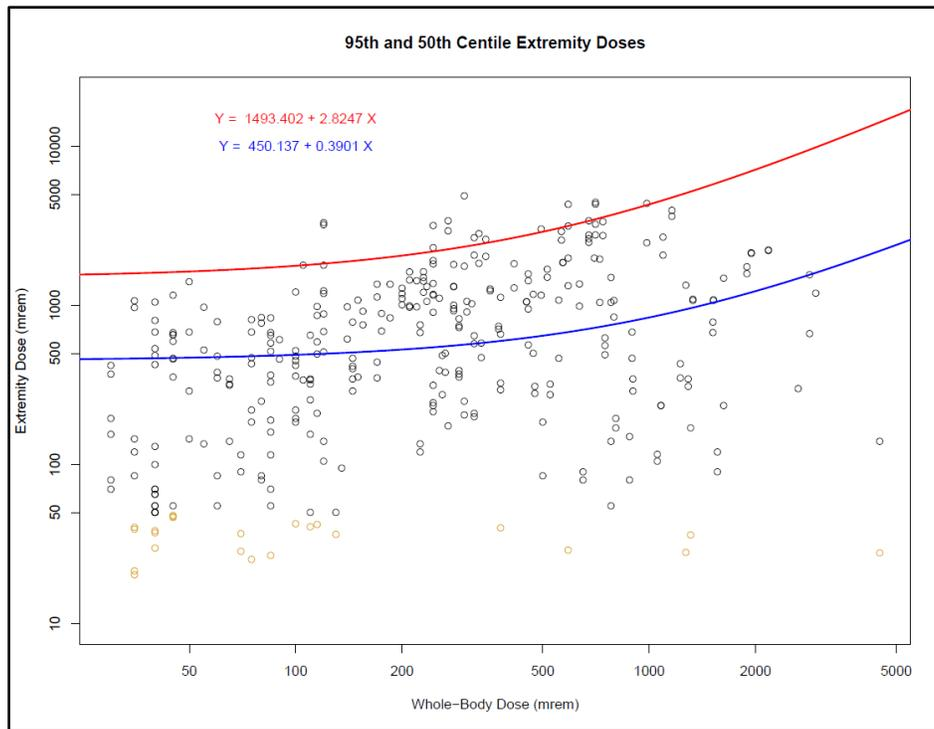
**Figure 2. Extremity Dose vs. Whole Body Dose with 50<sup>th</sup> and 95<sup>th</sup> Percentile Fit**
