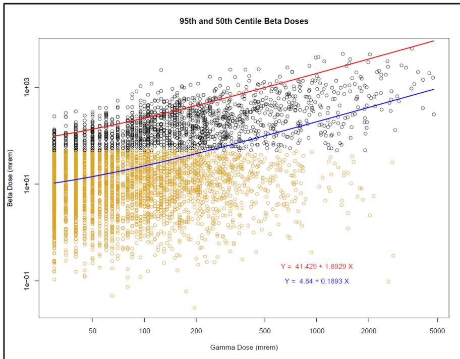
Figure 1. Beta Dose vs. Gamma Dose with 50<sup>th</sup> and 95<sup>th</sup> Percentile Fit
