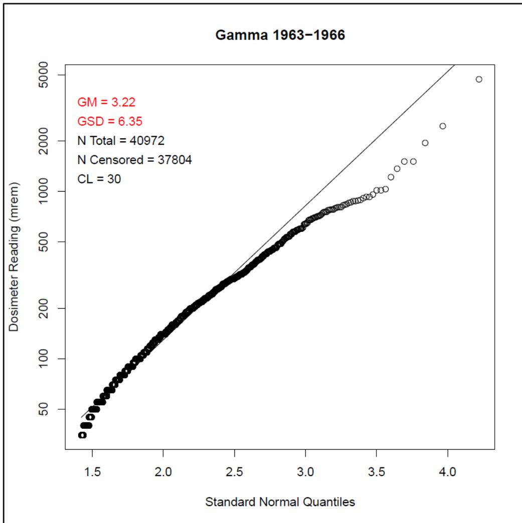
Figure 3. Imputation Model Results for NTS Photon Dose 1963–1966
