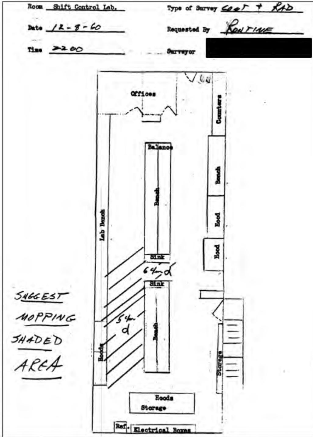
Figure 2: Contamination Survey of CPP Shift Control Lab in December 1960. (CPP 1960a, page 4)
