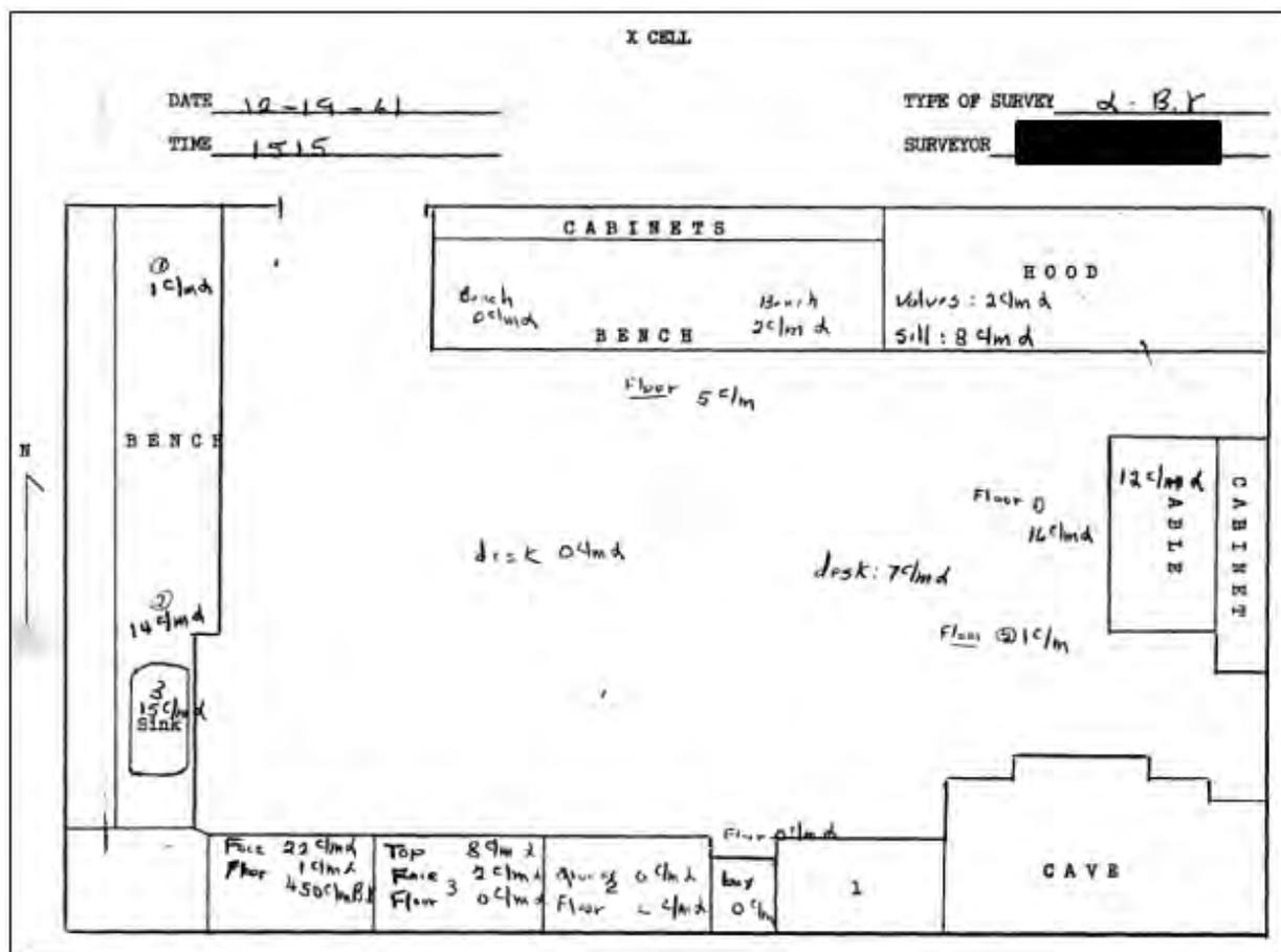
Figure 13: Contamination Survey of X-Cell in December 1961. Note the beta/gamma contamination level recording in the lower left hand corner. (CPP 1961a, page 6)
