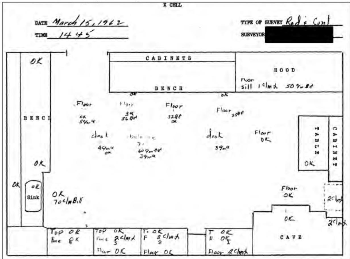
Figure 3: Contamination Survey of CPP X Cell in March 1962. (CPP 1962a, page 16)
