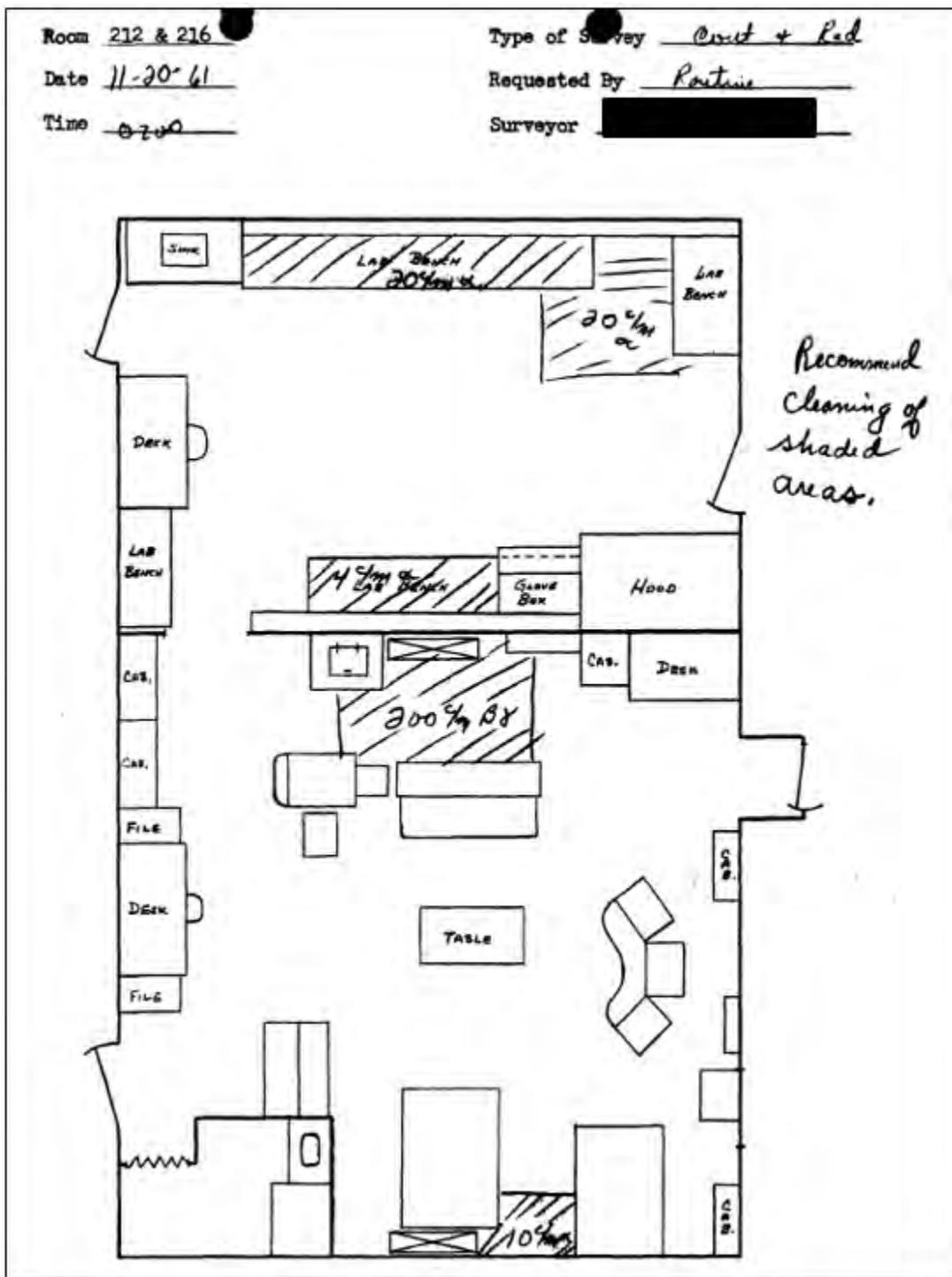
Figure 16: Alpha and Beta-Gamma Contamination Survey of CPP Labs 212/216 in November 1961. (CPP 1961b, page 24)
