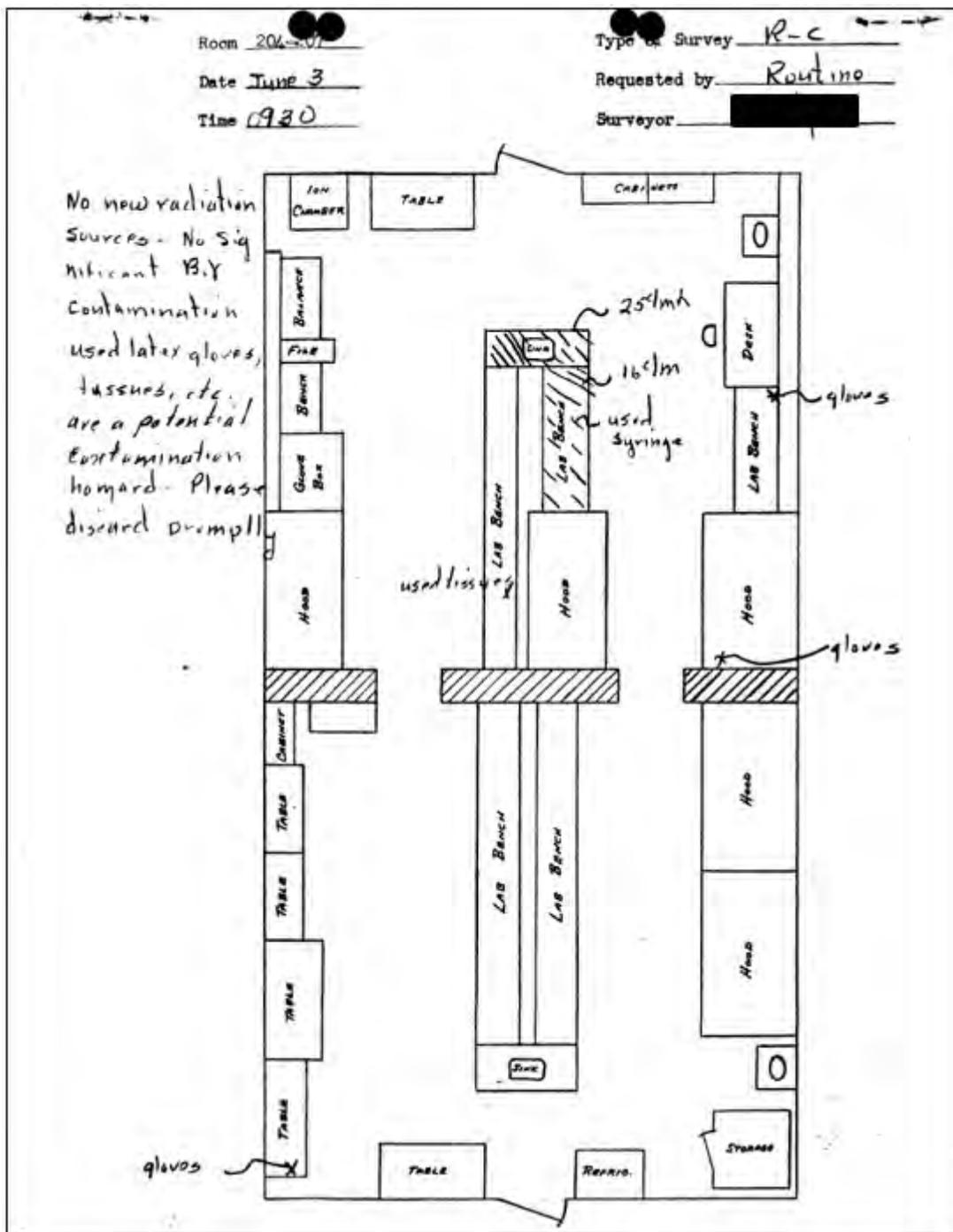
Figure 14: Contamination Survey of CPP Labs 204/207 in June 1961. Note the identification of potential sources of contamination on the survey. (CPP 1961a, page 6)
