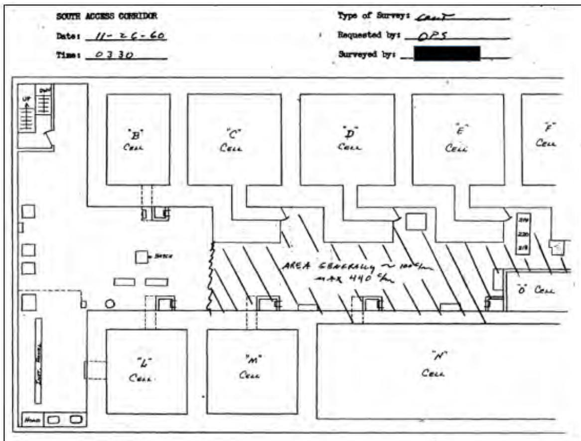
Figure 11: Beta-Gamma Contamination Survey of CPP-601 South Access Corridor (CPP 1960a, page 14)
