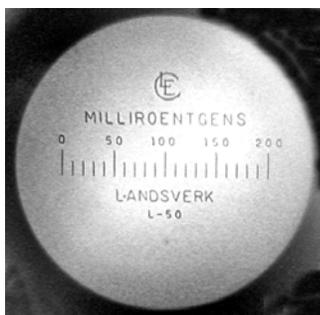
To use a pocket dosimeter, someone typically “zeros” the dosimeter using a charger before it is issued. The initial reading (ideally zero) is recorded and, at the end of the day, the dosimeter is read for the final reading. It can also be read at anytime during the day by the wearer. At the end of the day, the beginning reading (if not zero) is subtracted from the final reading to determine the dose received that day.
