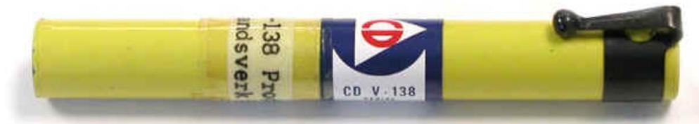
Figure 5 shows a drawing of a typical pocket dosimeter. The principle of the dosimeter is basically that of an electroscope. A charge is put on the fibers where one fixed and one movable fiber repel each other. As ionizing radiation ionizes the air in the chamber, the charge is collected on the fibers and they repel each other a little less. As the charge is lessened, the movable fiber casts a shadow across a scale showing a higher dose.
