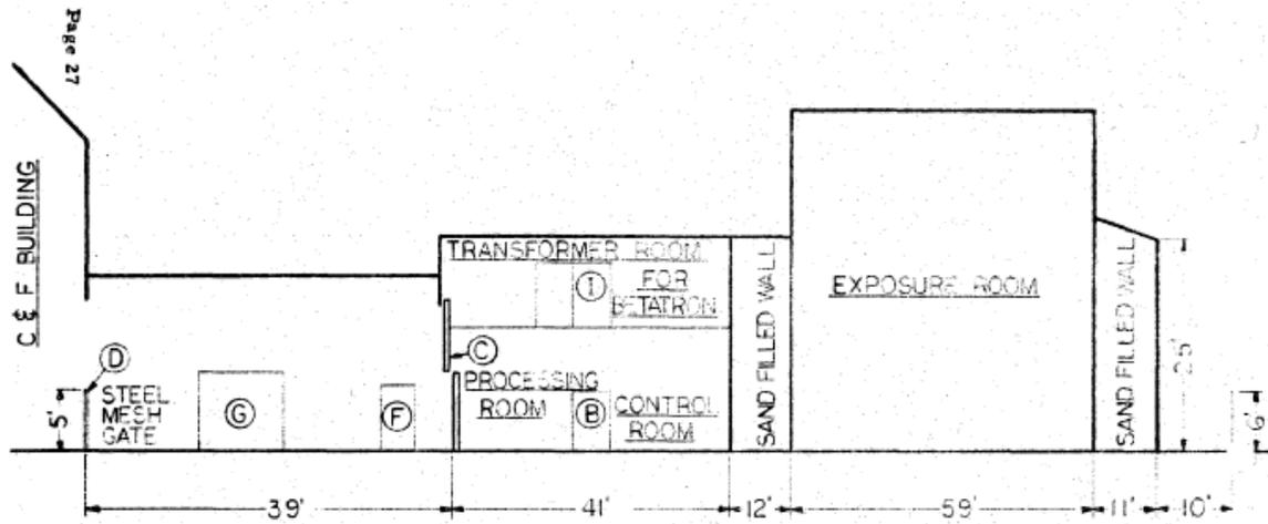
A survey of the new betatron building with an 80 curie cobalt-60 source exposed was conducted on January 29, 1971 (ML093480290). The survey, which included measurements taken at various points around the building, is reproduced in Table 1. The letters in parentheses correspond to the locations identified in Figures 2 through 4.
