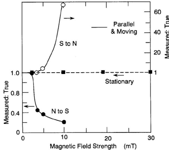
Fig. 4. Response of the Victoreen 450p ion chamber survey meter. True signal is  $0.77 \mu\text{C kg}^{-1} \text{h}^{-1}$  ( $3 \text{ mR h}^{-1}$ ).
