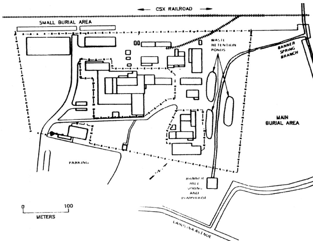
**Figure 5: Layout of the NFS plant showing waste burial areas (ORAU, 1987, pdf p. 29)**
