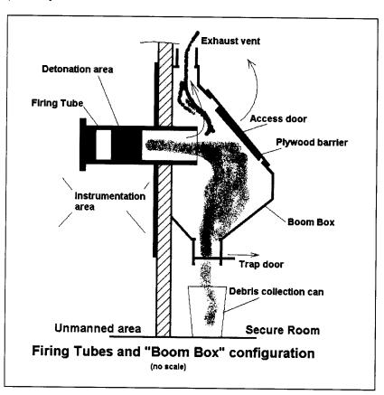
The boom box was actually one large welded unit and had a permanent steel barrier between each compartment.
