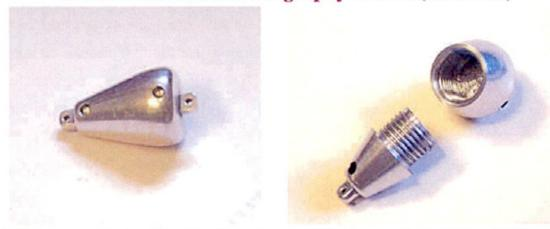
This is an example of an industrial radiography source of the type used in the 1930s and 1940s. Sometimes referred to as a plumbbob, it would have contained approximately 0.1 Ci of Ra-226. Although expensive, radium was used because no other radionuclides were then available of sufficient strength. After World War II, Ir-192 and Co-60 quickly became the radionuclides of choice and the use of radium was abandoned.
