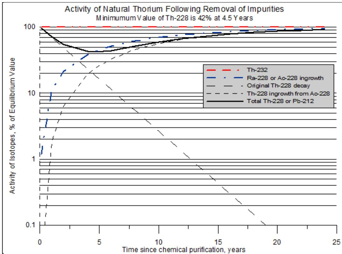
Figure 5-1. Decay and buildup of  $^{228}\text{Th}$  and daughters following processing.
