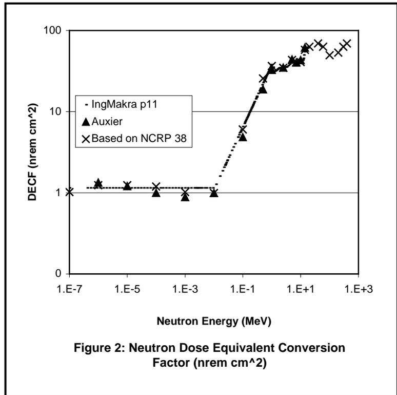
Figure 2: Neutron Dose Equivalent Conversion Factor (nrem cm<sup>2</sup>)
