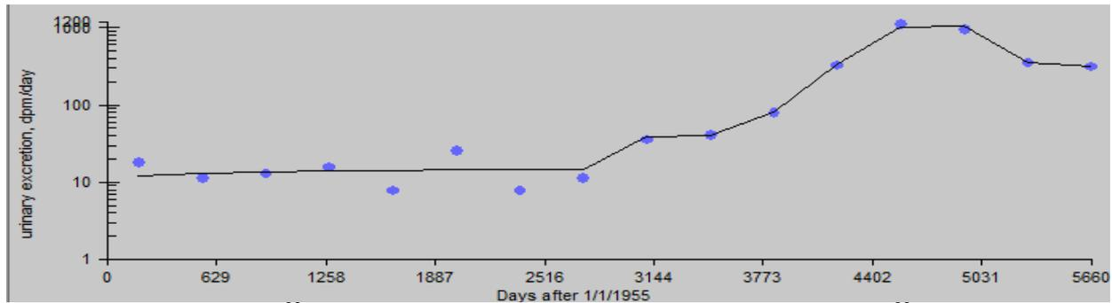
Figure B-76. Predicted  $^{60}\text{Co}$  bioassay results calculated using IMBA-derived  $^{60}\text{Co}$  intake rates (line) compared with bioassay results (dots), 50th percentile, type S.
