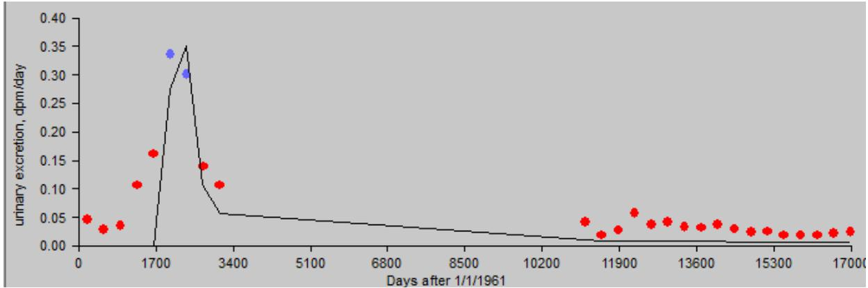
Figure B-58. Predicted neptunium bioassay results calculated using IMBA-derived neptunium intake rates (line) compared with bioassay results (dots), 84th percentile, 1966–1967, type M.
