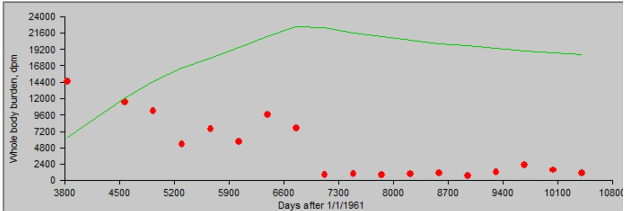
Figure B-67. Predicted neptunium bioassay results calculated using IMBA-derived neptunium intake rates (line) compared with bioassay results, 84th percentile, 1961–2007 cumulative, type M, urinalysis data, whole-body count data.
