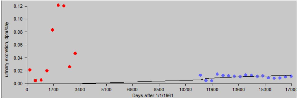
Figure B-55. Predicted neptunium bioassay results calculated using IMBA-derived neptunium intake rates (line) compared with bioassay results (dots), 50th percentile, 1991–2007, type M.
