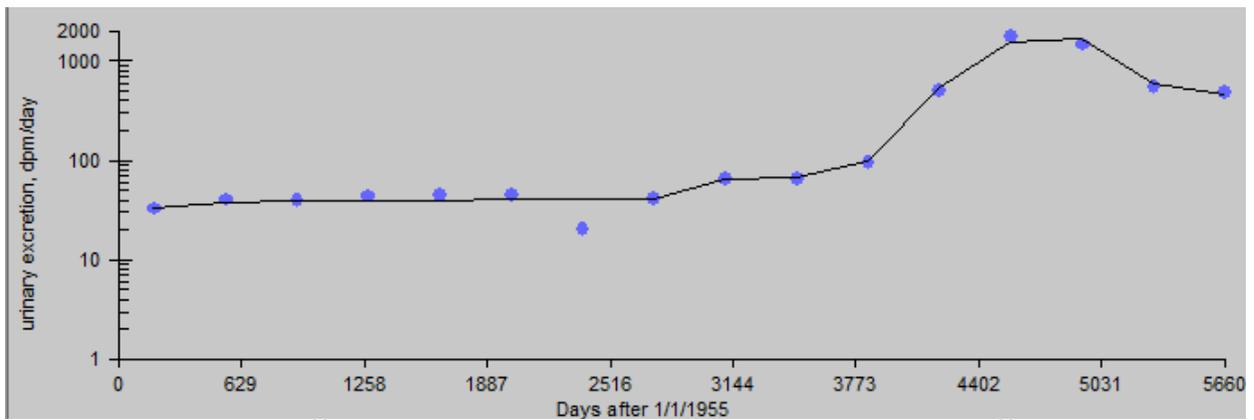
Figure B-75. Predicted  $^{60}\text{Co}$  bioassay results calculated using IMBA-derived  $^{60}\text{Co}$  intake rates (line) compared with bioassay results (dots), 84th percentile, type M.
