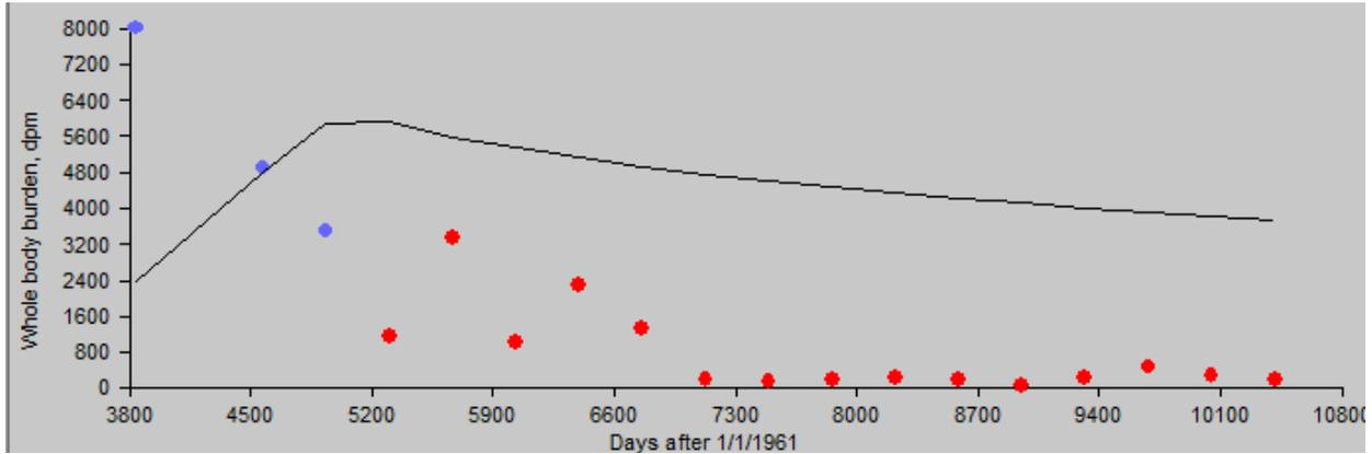
Figure B-52. Predicted neptunium bioassay results calculated using IMBA-derived neptunium intake rates (line) compared with bioassay results (dots), 50th percentile, 1970–1974, type M.
