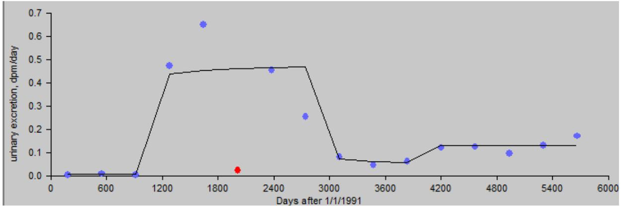
Figure B-69. Predicted strontium bioassay results calculated using IMBA-derived strontium intake rates (line) compared with bioassay results (dots), 50th percentile, 1991–2006, type F.
