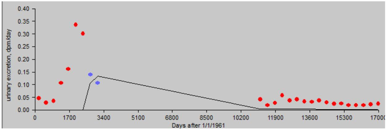
Figure B-59. Predicted neptunium bioassay results calculated using IMBA-derived neptunium intake rates (line) compared with bioassay results (dots), 84th percentile, 1968–1969, type M.
