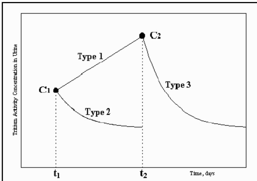
Figure 4-1. Diagram from ORAUT-OTIB-0011 that shows the types of methods used to determine the area under an excretion curve.
