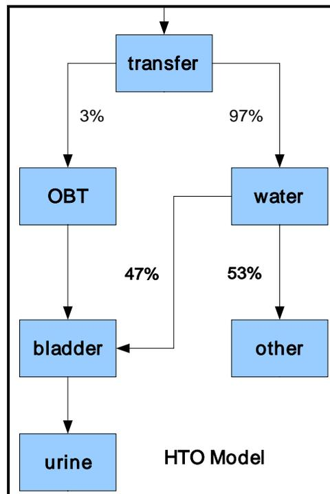
Figure 3-1. Biokinetic model for HTO.
