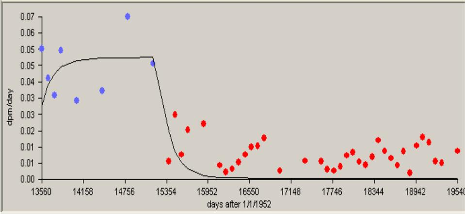
Figure B-5. Predicted uranium bioassay results (line) calculated using IMBA-derived U intake rates compared with measured uranium-in-urine results (dots), 1/1/1989 to 12/31/1993, 50th-percentile, Type M.
