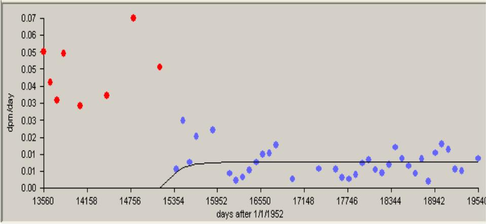
Figure B-6. Predicted uranium bioassay results (line) calculated using IMBA-derived U intake rates compared with measured uranium-in-urine results (dots), 1/1/1994 to 12/31/2005, 50th-percentile, Type M.
