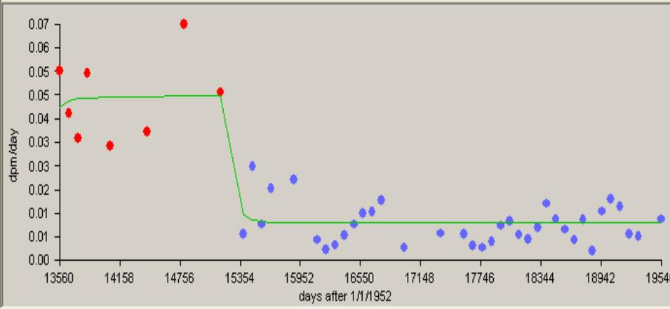
Figure B-3. Predicted uranium bioassay results (line) calculated using IMBA-derived U intake rates compared with measured uranium-in-urine results (dots) from all intakes 1/1/1989 to 12/31/2005, 50th-percentile, Type F.
