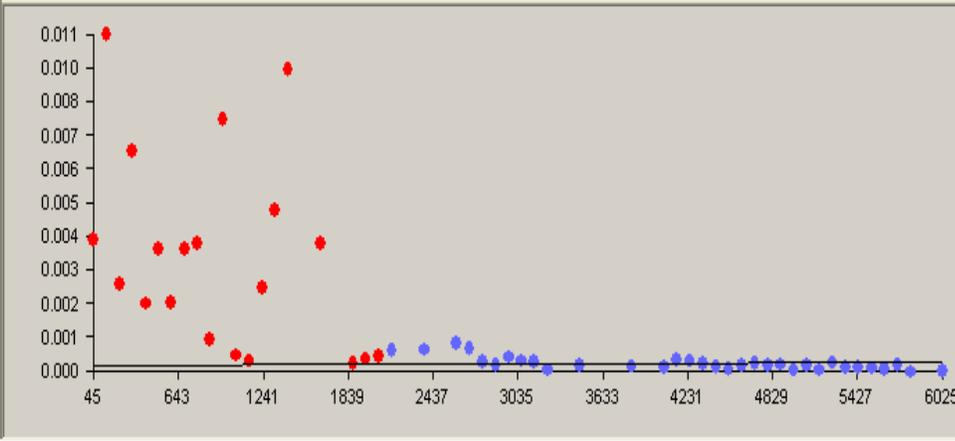
Figure B-17. Predicted plutonium bioassay results (line) calculated using IMBA-derived Pu intake rates compared with measured Pu-in-urine results (dots), 1/1/1952 to 12/31/2005, 50-percentile, Type S.
