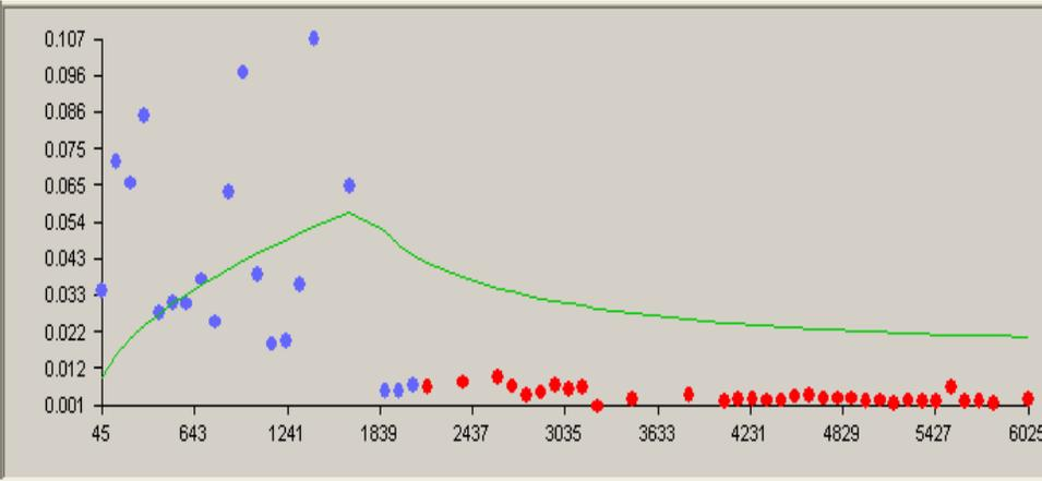
Figure B-16. Predicted plutonium bioassay results (line) calculated using IMBA-derived Pu intake rates compared with measured Pu-in-urine results (dots), 1/1/1989 to 12/31/2005, 84th-percentile, Type M.
