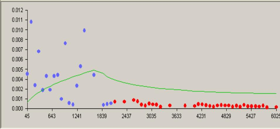
Figure B-15. Predicted plutonium bioassay results (line) calculated using IMBA-derived Pu intake rates compared with measured Pu-in-urine results (dots), 1/1/1989 to 12/31/2005, 50th-percentile, Type M.
