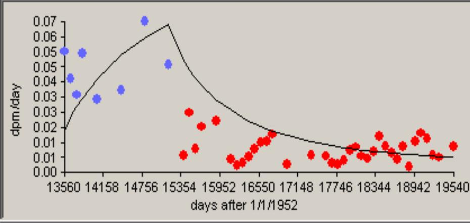
Figure B-9. Predicted uranium bioassay results (line) calculated using IMBA-derived U intake rates compared with measured uranium-in-urine results (dots), 1/1/1989 to 12/31/1993, 50th-percentile, Type S.
