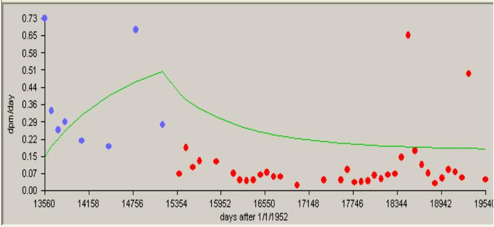
Figure B-12. Predicted uranium bioassay results (line) calculated using IMBA-derived U intake rates compared with measured uranium-in-urine results (dots), 1/1/1989 to 12/31/2005, 84th-percentile, Type S.
