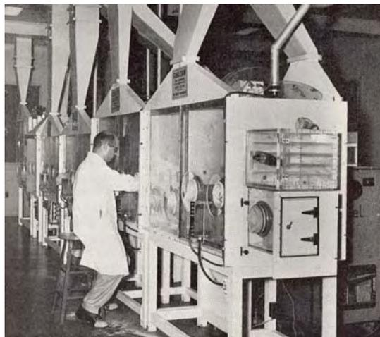
Figure 2 Plutonium gloveboxes at Chalk River <sup>(1)</sup>
