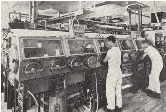
Figure 1 Plutonium gloveboxes at LANL <sup>(1)</sup>
