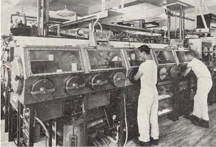
Figure 1 Plutonium gloveboxes at LANL <sup>(1)</sup>
