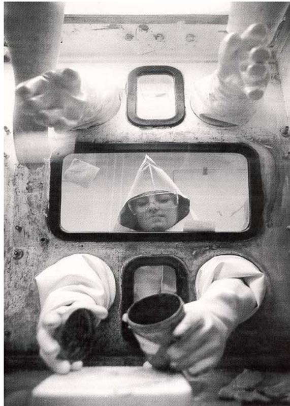
Figure 5 Other plutonium gloveboxes at Hanford. Note the viewing area in direct line with the lower torso in the center between the gloves.<sup>(2)</sup>
