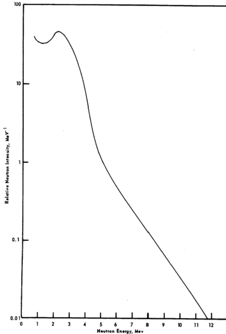
Figure 6-2.<sup>a</sup> RTG Plutonium Source Neutron Energy Spectrum – PuO<sub>2</sub> Microspheres.
