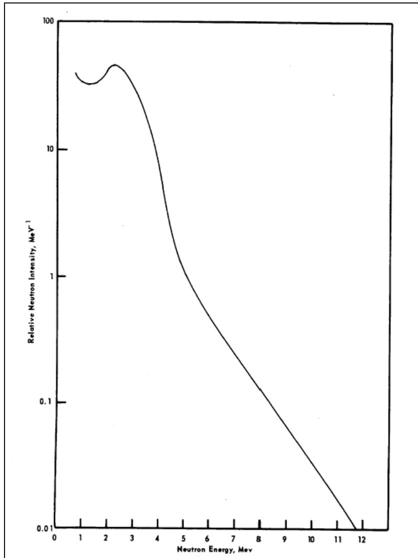
Figure 6-2. RTG Plutonium Source Neutron Energy Spectrum – PuO<sub>2</sub> Microspheres.<sup>a</sup> a. (Burkhart, 1987a)
