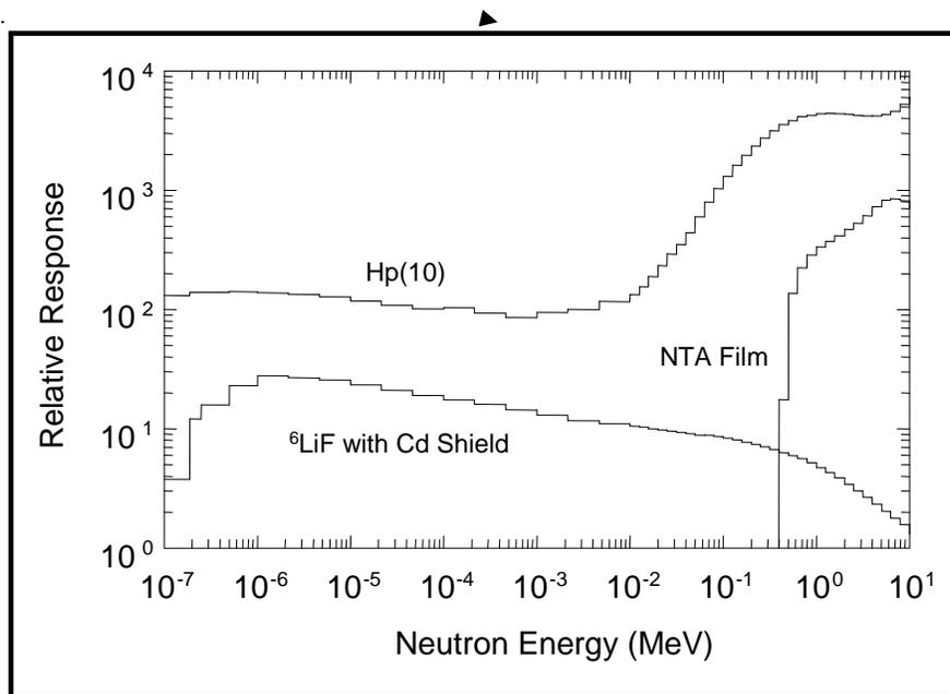
Figure 6-4. Comparison of  $Hp(10)$  from normally incident neutrons to energy responses of NTA film and neutron albedo dosimeter containing neutron TLD chip made of  ${}^6\text{LiF}$  and shielded by cadmium (IAEA 1990).
