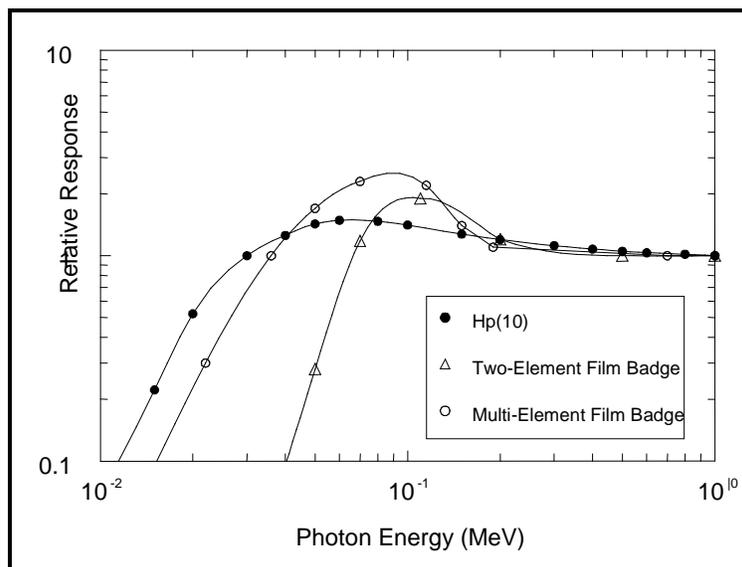
Figure 6-2. Comparison of  $Hp(10)$  for photons with energy responses for sensitive DuPont 502 emulsion in MED two-element film badge (Pardue, Goldstein, and Wollan 1944) and sensitive DuPont 555 emulsion in Oak Ridge National Laboratory multielement film badge (Thornton, Davis, and Gupton 1961).
