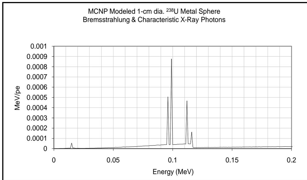
Figure 6-8. Characteristic X-ray component of calculated spectrum from <sup>238</sup>U spheres on linear vertical axis. Source: Calculations made using Los Alamos 2003.
