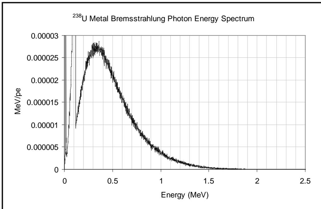
Figure 6-7. *Bremsstrahlung* component of calculated spectrum from  $^{238}\text{U}$  spheres on linear vertical axis. Source: Calculations made using Los Alamos 2003.
