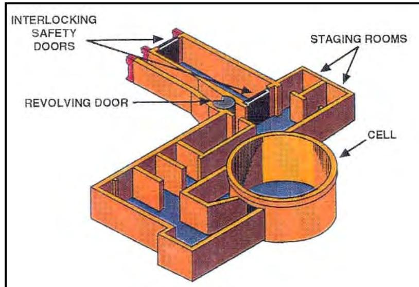
Figure 2-5. Generic representation of a nuclear explosive cell.
